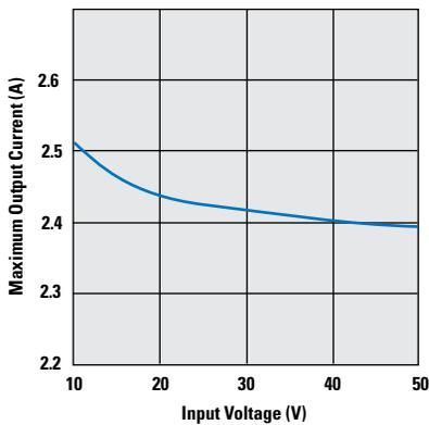
**Figure 4. Maximum Output Current vs Input Voltage**
