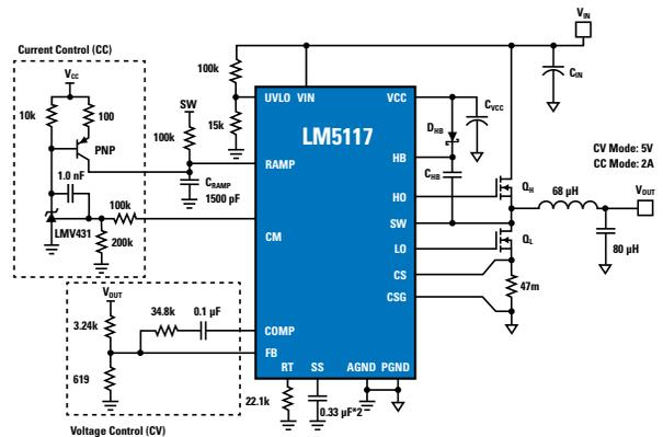
**Figure 8. Constant Voltage Regulator with Precision Current Limit**
