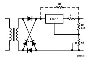
FIGURE 1. Constant Voltage Charging Circuit
