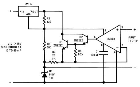
Figure 8. 10 mA to 50 mA 2-Wire Current Transmitter
