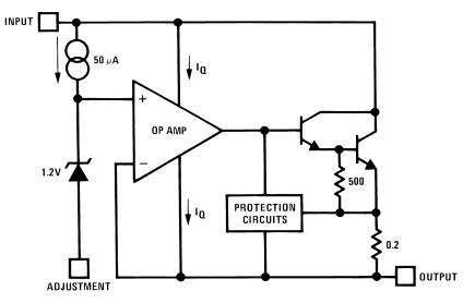
Figure 1. Functional Schematic of the LM117
