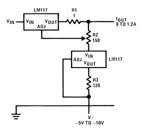
Figure 7. Adjustable Current Regulator
