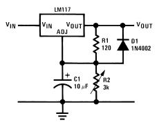
Figure 2. Basic Voltage Regulator
