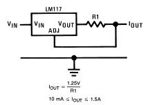
Figure 5. 2-Terminal Current Regulator
