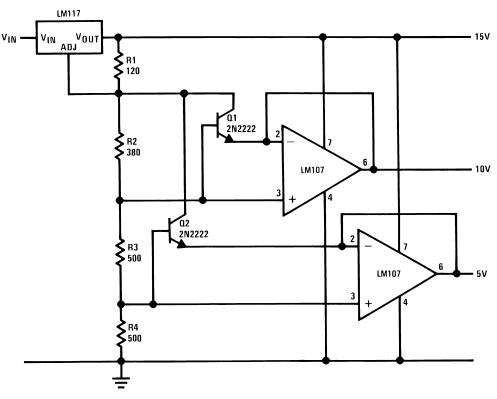
Figure 4. Regulator with Multiple Outputs
