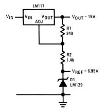
Figure 3. Regulator and Voltage Reference
