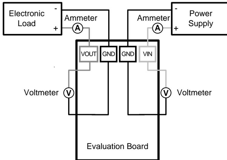
Figure 4. Efficiency Measurements
