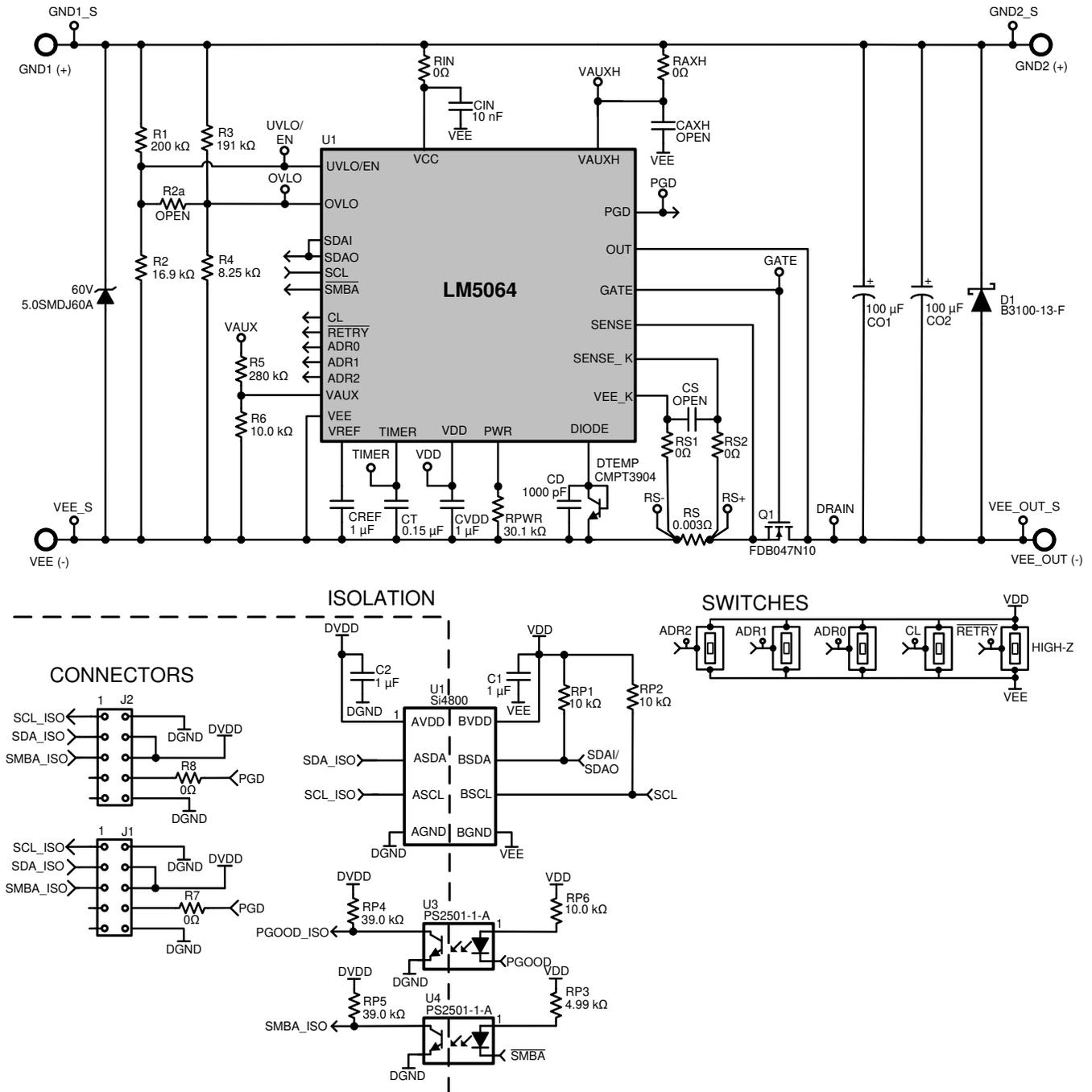
Figure 2. Full Evaluation Board Schematic
