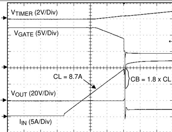
Figure 17. Circuit Breaker Event (CL = VDD) 4 ms/div
