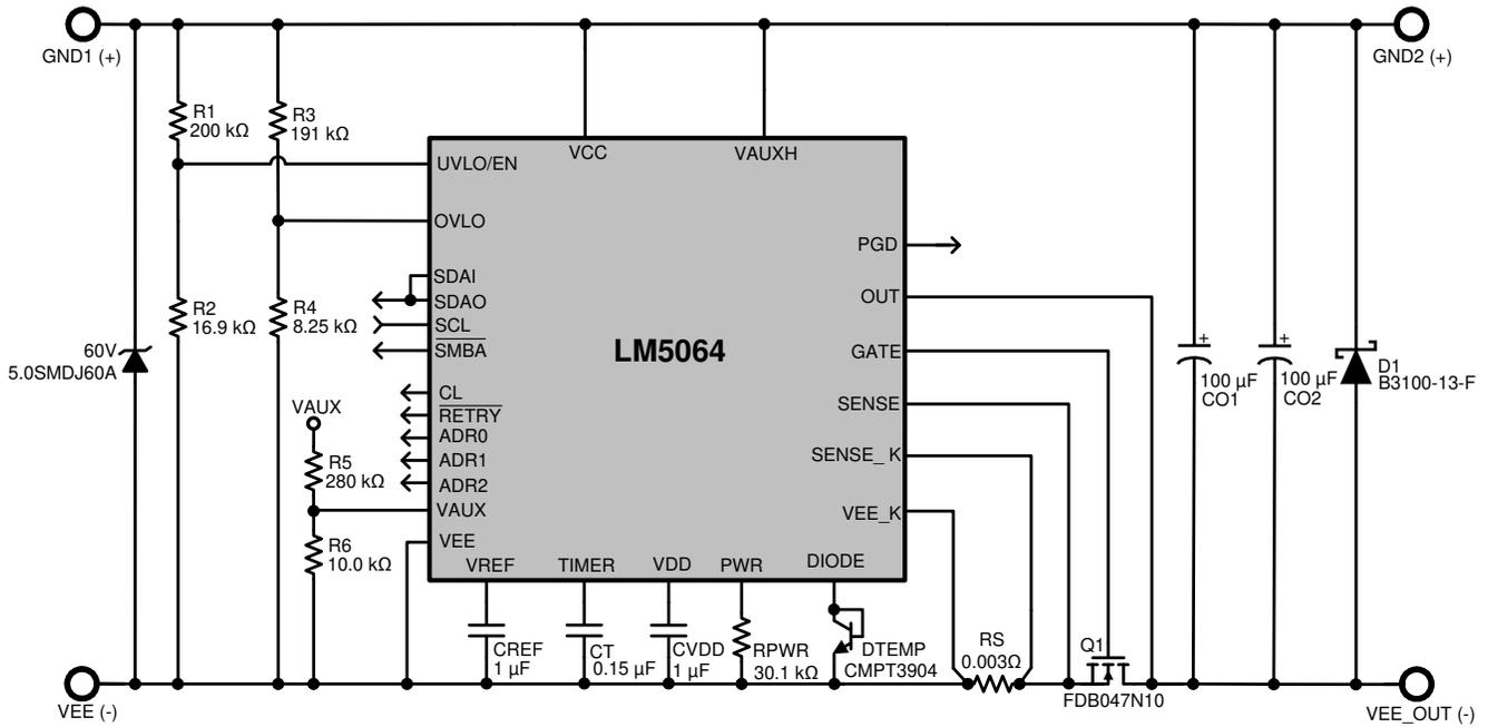
Figure 1. Simplified Schematic
