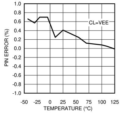
**Figure 22. PIN Error vs Temperature**
