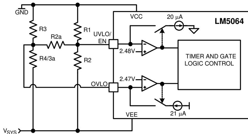
Figure 14. Programming the UVLO and OVLO Thresholds
