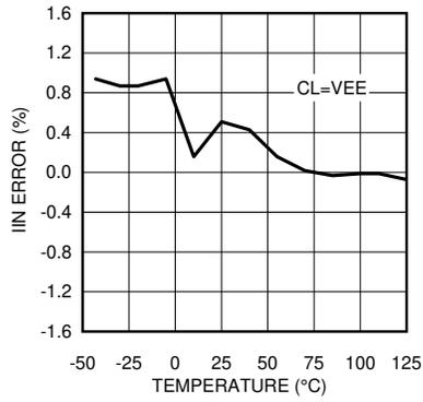
**Figure 21. IIN Error vs Temperature**
