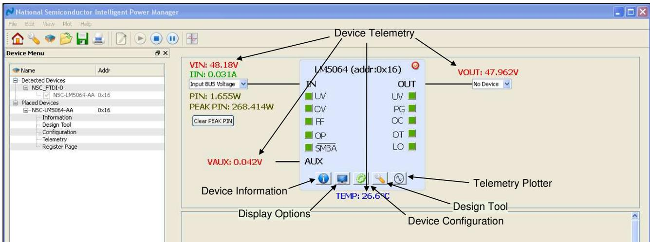
Figure 6. LM5064 Block Level Representation
