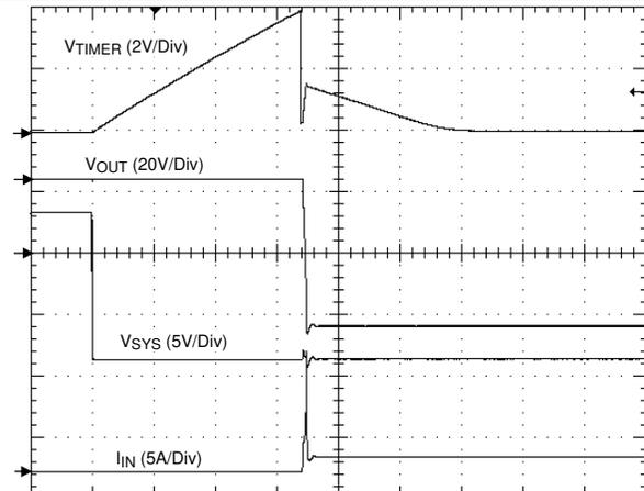
Figure 16. Turn-On Sequence into a 40Ω Load (40 ms/div)
