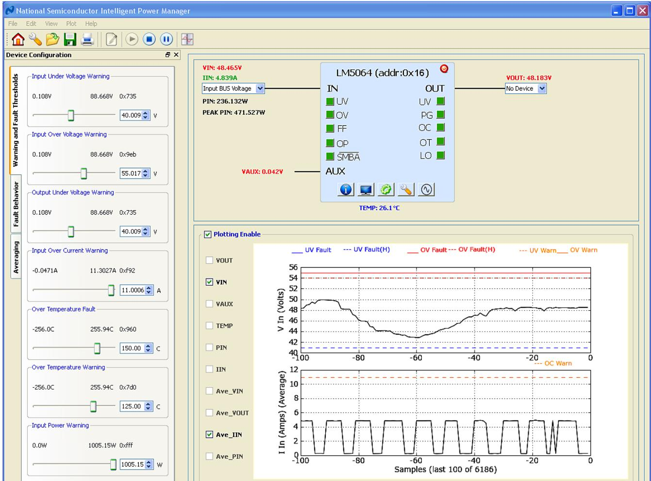
Figure 8. LM5064 GUI with Telemetry Plotting Tool Enabled
