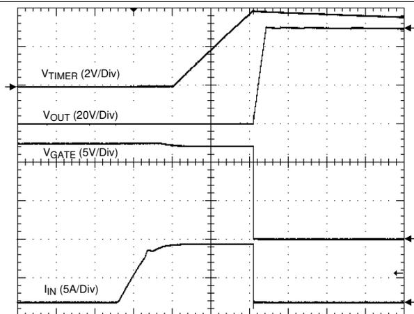
Figure 18. Current Limit Event (CL = VDD) 4 ms/div
