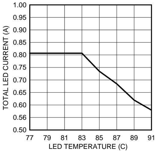
**Figure 4. Total LED Current vs. LED Temperature**
