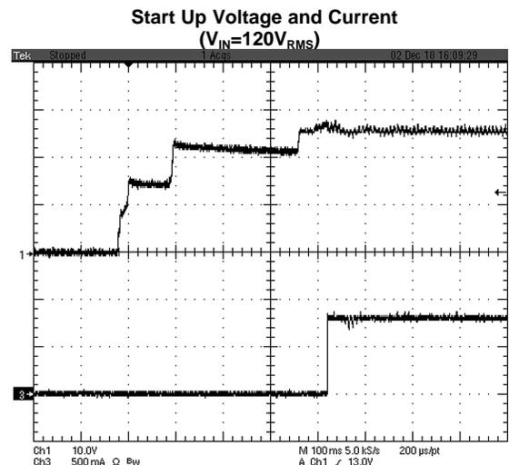
Figure 9. Ch1: Output Voltage (10 V/div);
