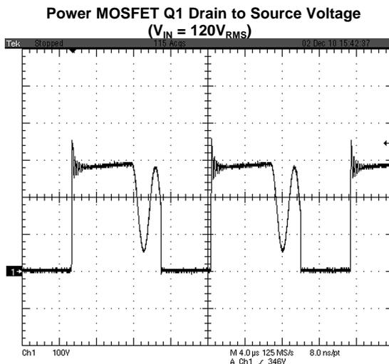
Figure 8. Ch1: Drain Voltage (100V/div)
