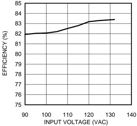
**Figure 2. Efficiency vs. Line Voltage**
