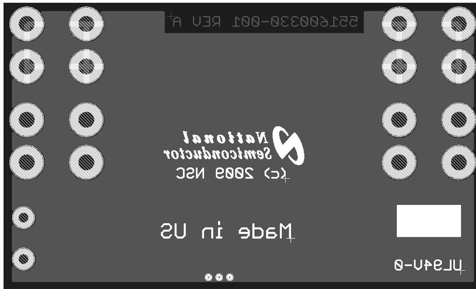
**Figure 10. Evaluation Board, Bottom Side**
