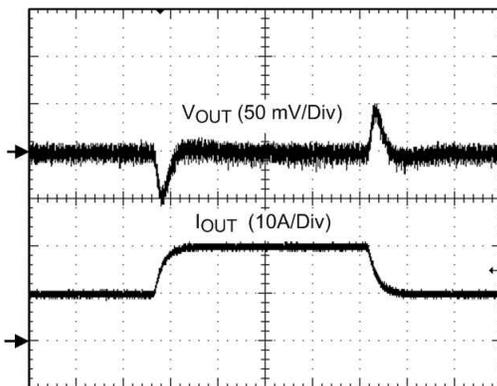
**Figure 6-5. 10-A to 20-A Load Transient Response**
