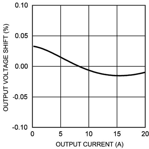
**Figure 6-3. Load Regulation ( $V_{IN} = 12\text{ V}$ )**
