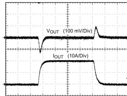
**Figure 6-6. 0-A to 20-A Load Transient Response**
