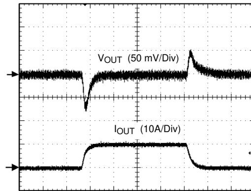
**Figure 6-4. 0-A to 10-A Load Transient Response**
