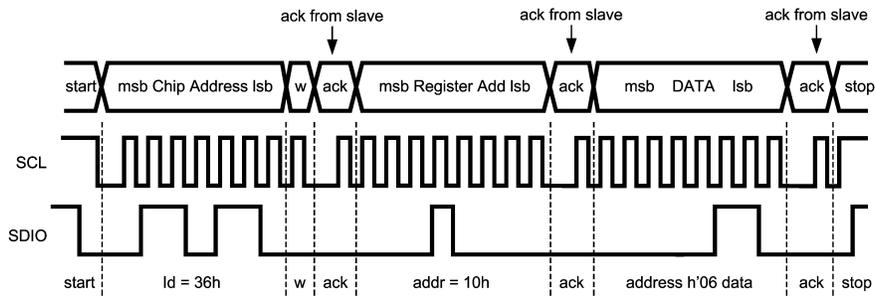
NOTE: w = write (SDIO = "0"); r = read (SDIO = "1"); ack = acknowledge (SDIO pulled down by either master or slave); id = chip address, 36h for LM27965
