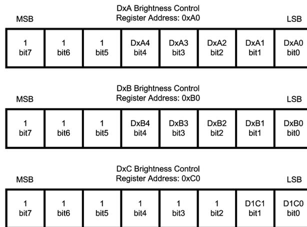
**Figure 8. Brightness Control Register Description**
