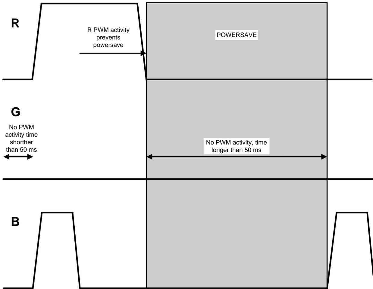
Figure 2. Basic Power Save Sequence With Long Inactive Period
