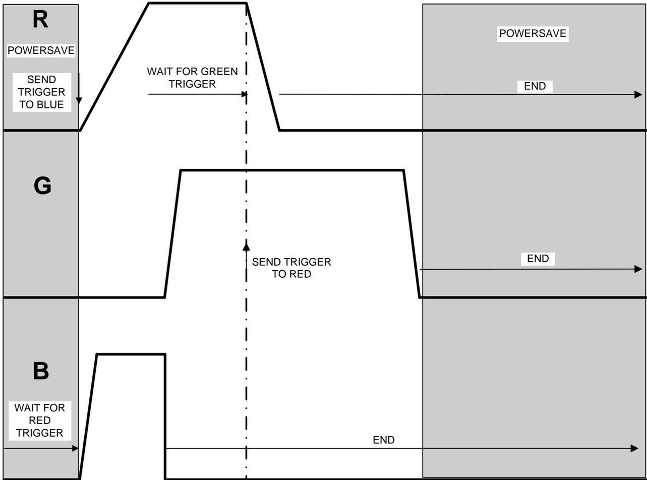
Figure 4. Power Save Sequence With Wait for Trigger Command
