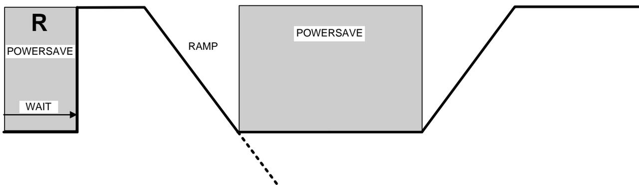
Figure 3. Power Save Sequence With a Ramp Command Used as Combined Ramp/Wait
