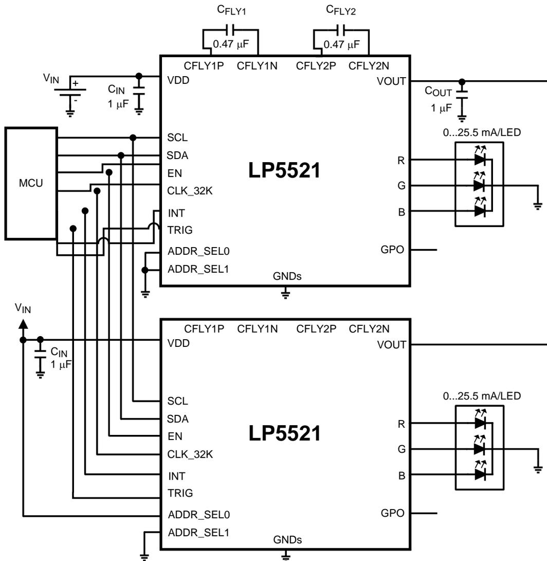
Figure 1. One LP5521 is Supplying Two  $V_{OUTs}$
