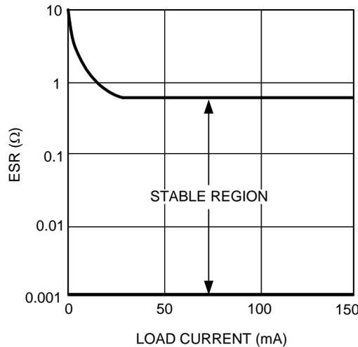
**Figure 7. C<sub>OUT</sub> ESR Stability Boundaries for Typical "Ceramic Stable" LDO**
