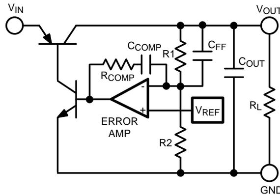
Figure 5. Ceramic-Stable LDO With Internal Compensation Zero
