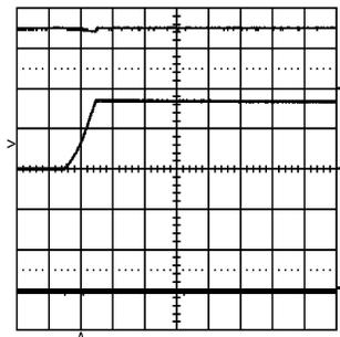
Trace 1: Input Voltage, at 30VDC. Volts/div = 20.0V Trace 2: Output Voltage, no load. Volts/div = 2.0V Trace 3: Output Current, no load. Amps/div = 100mA Horizontal Resolution = 1.0ms/div
