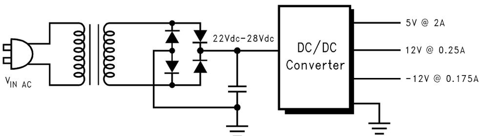
**Figure 7. 3-Output Flyback Converter Provides Power for Modem**
