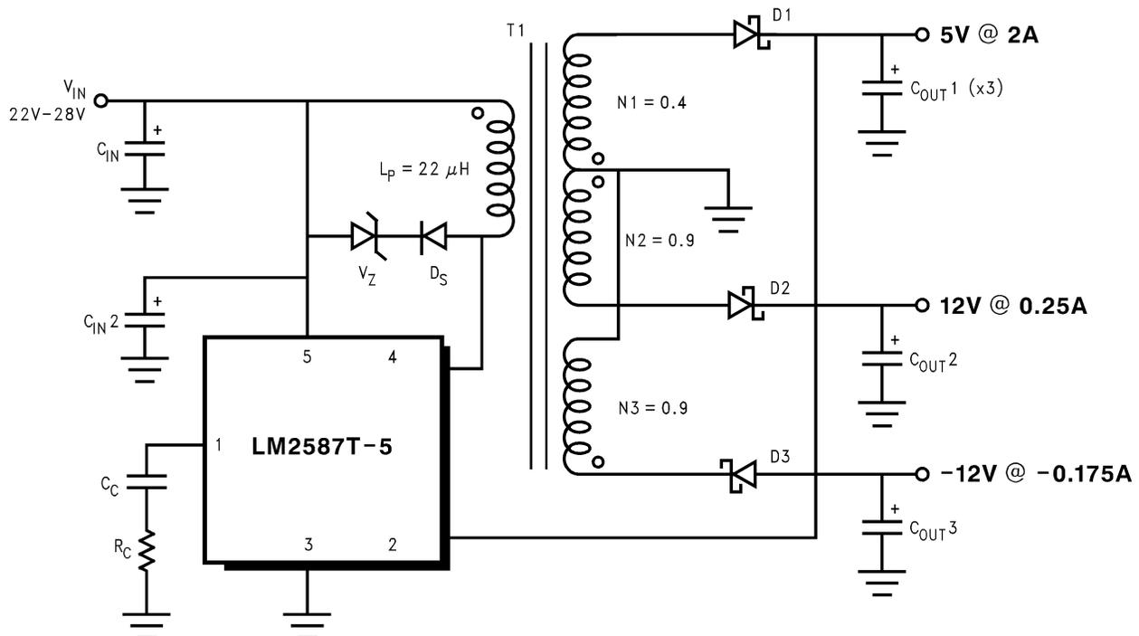
Figure 8. Schematic for Power Supply of Figure 7
