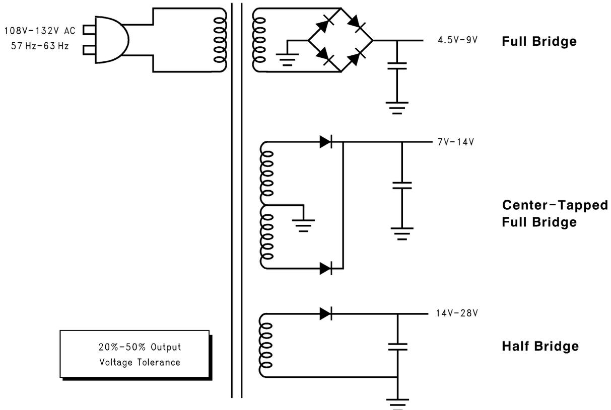
Figure 3. AC Line Rectification Methods
