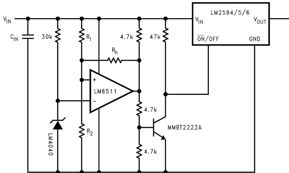
Figure 10. Undervoltage Lockout Circuit with Hysteresis
