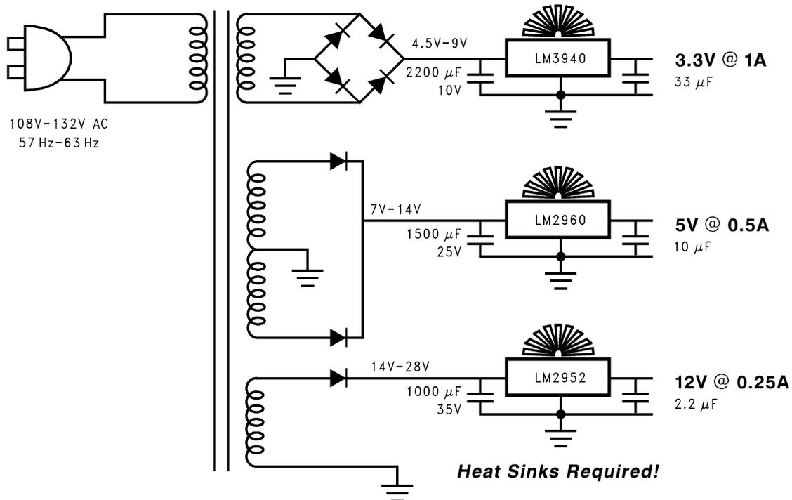
Figure 5. Power Supply Solution Using Linear Regulators
