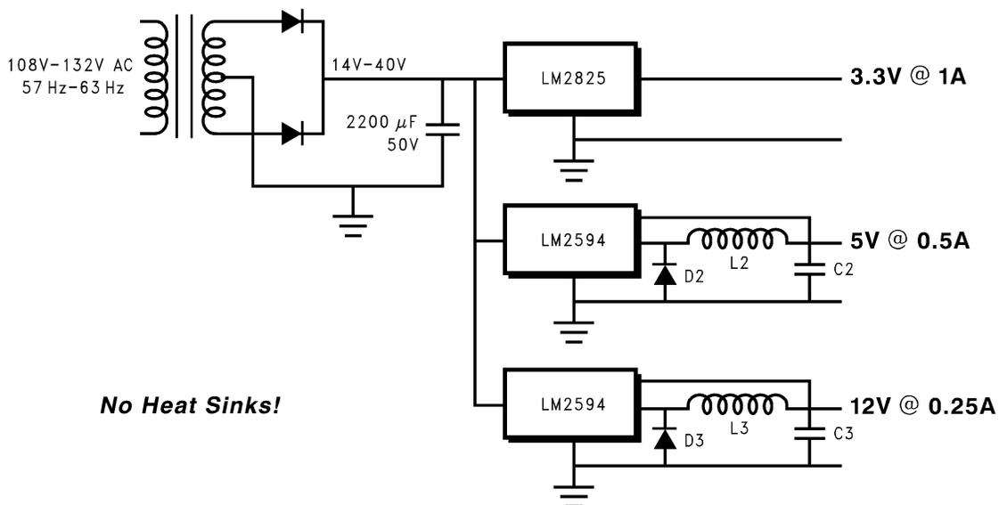
Figure 6. Power Supply Solution Using Step-Down Switching Regulators
