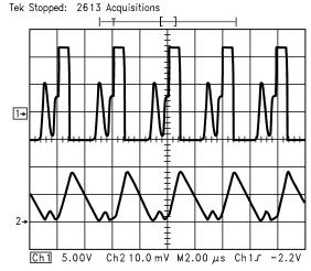
Upper Trace: Switch Voltage, 5V/div Lower Trace: Inductor Current, 0.5A/div Horizontal: 2µs/div
