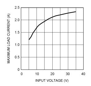
Figure 5. LM2673 Input Voltage vs. Load Current ( $V_{out} = -5 V$ , L = 33µH)
