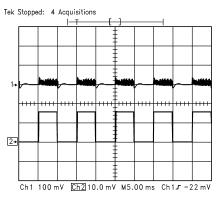
Upper Trace: Output Voltage, 100m V/div Lower Trace: Load Current, 1A/div Horizontal: 2µs/div
