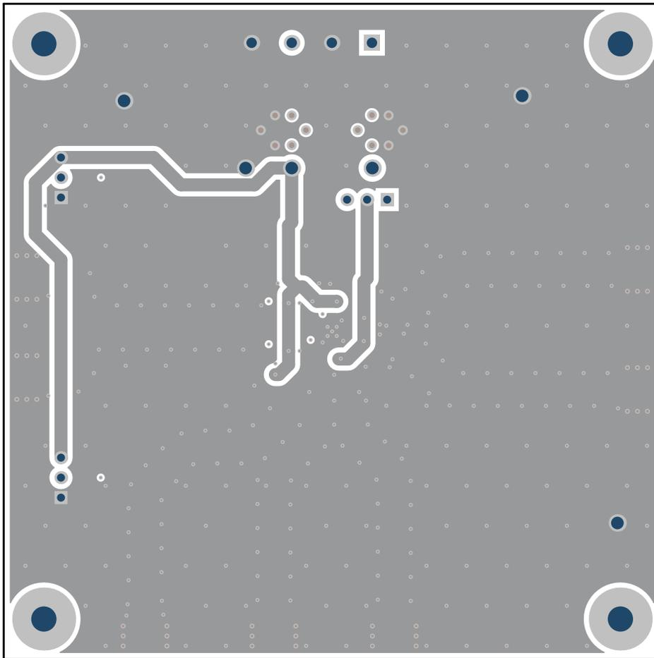
**Figure 4. Inner Layer 3 (VDD Traces and GND Fill)**
