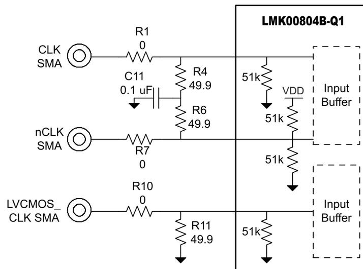
Figure 1. On-Board Input Termination With Internal Pullup/Pulldown Resistors
