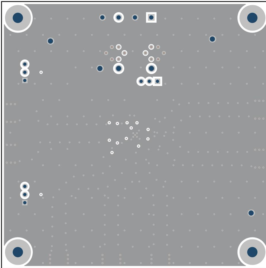
**Figure 3. Inner Layer 2 (Ground Plane)**
