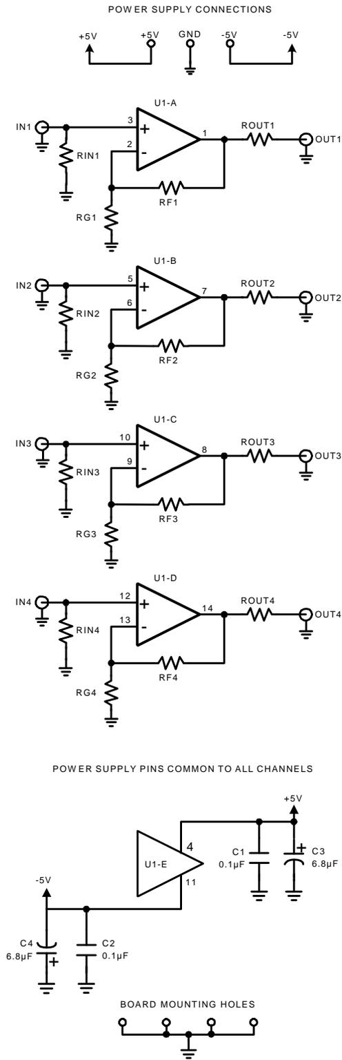
**Figure 1: Non-Inverting Op Amp Configuration
