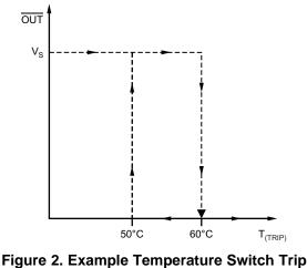
Figure 2. Example Temperature Switch Tr Behavior With Hysteresis
