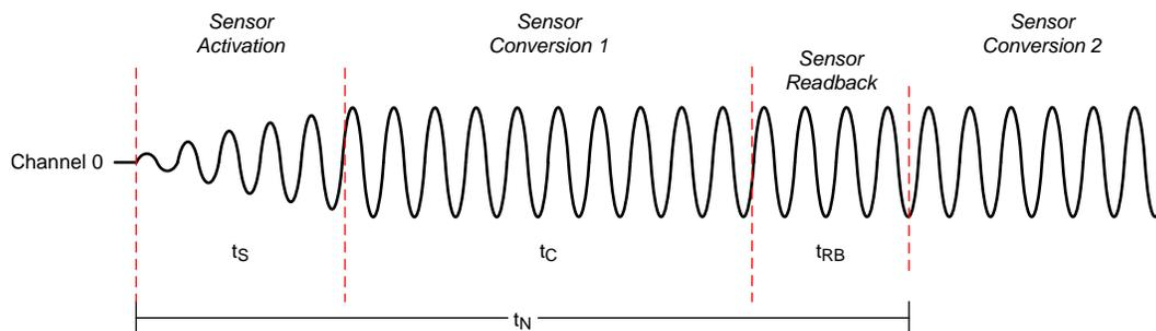
**Figure 1. Single Channel Mode Sequencing in Continuous Conversion**
