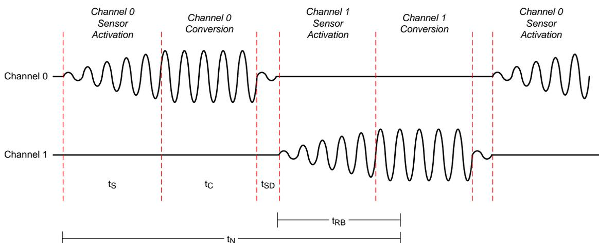
**Figure 2. Multi-Channel Mode Sequencing in Continuous Conversion**
