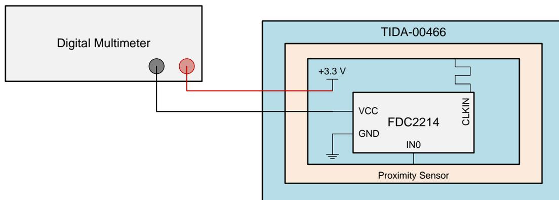
**Figure 4. Test Setup**
