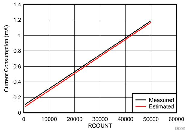
Figure 5. Comparison Between Measured and Estimated Current Consumption
