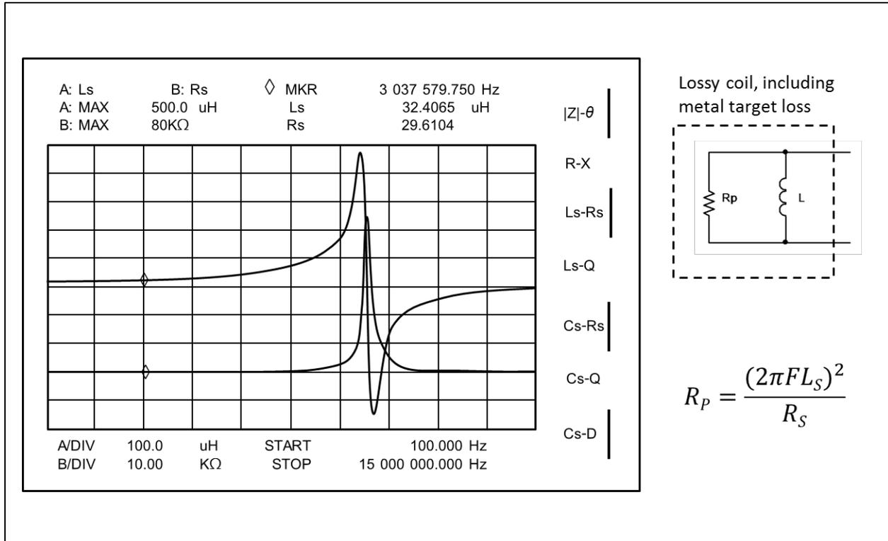
**Figure 2. Using an Impedance Analyzer to Find R<sub>p</sub>.**
