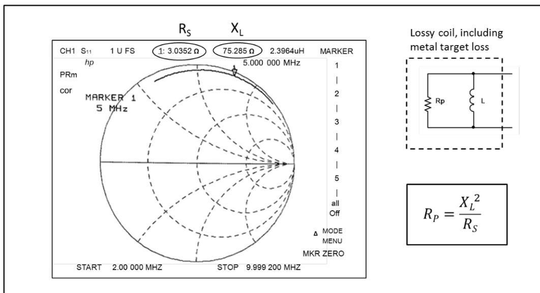
**Figure 1. Using a Network Analyzer to Find  $R_p$ .**
