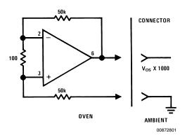
FIGURE 1. Drift Measurement Circuit
