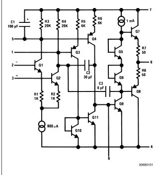
FIGURE 1. Simplified Circuit of the LM118
