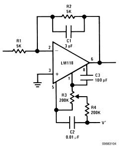
†Slew and settling time to 0.1% for a 10V step change is 800 ns.
