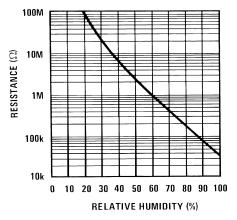
Figure 1. Phys-Chemical Research Corp. Model PCRC-55 Humidity Sensor
