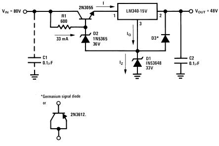
Figure 21. High Voltage Regulator
