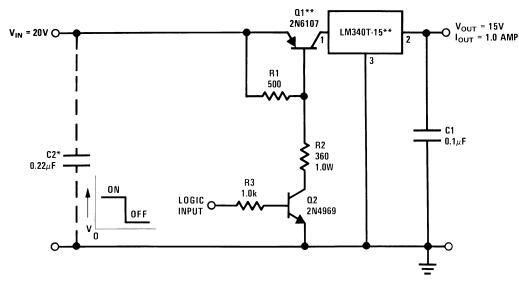
\*Required if the regulator is located far from the power supply filter \*\*Head sink Q1 and the LM340
