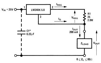
\*Required if regulator is located far from power supply filter
