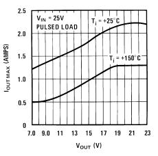
Figure 13. Maximum Output Current
