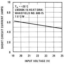
Figure 8. Continuous Short Circuit Current vs Input Voltage
