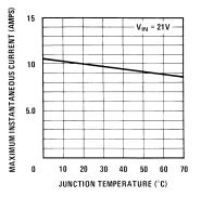
Figure 7. Maximum Instantaneous Current vs Junction Temperature
