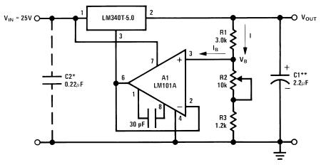
\*Required if the regulator is located far from the power supply filter \*\*Solid tantalum
