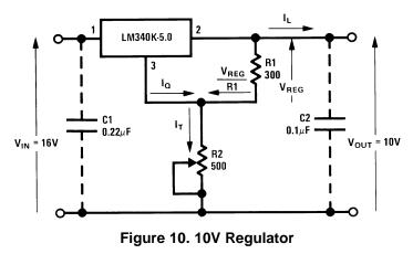
The 5.0V pedestal results from the sum of regulator quiescent current  $I_{Q}$  and a current equal to  $V_{REG}/R1$ , flowing through potentiometer R2 to ground. R2 is made adjustable to compensate for differences in  $I_{Q}$  and  $V_{REG}$  output. The circuit is practical because the change in  $I_{Q}$  due to line voltage and load current changes is quite small.
