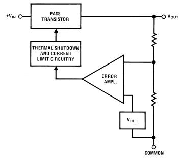
Figure 1. Functional Block of the LM340
