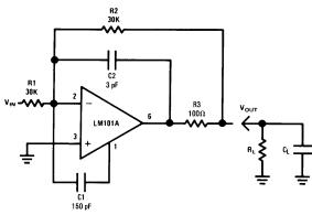
Figure 7. Capacitive load isolation
