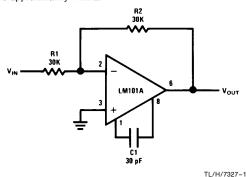
Figure 1. Standard frequency compensation
