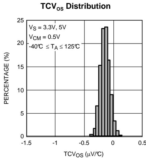
**Figure 2. Percentage vs. TCV<sub>OS</sub> Distribution for LMP7731 (Typical Characteristics)**
