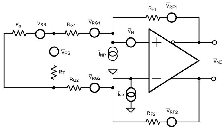
Figure 2. Fully Differential Amplifier Noise Model
