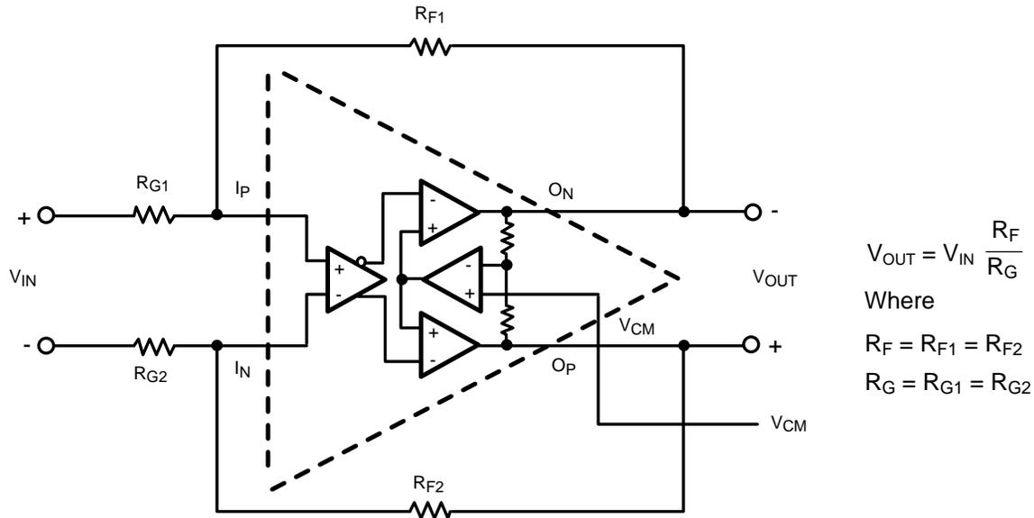
**Figure 1. Simplified Conceptual Diagram of Fully Differential Amplifier**
