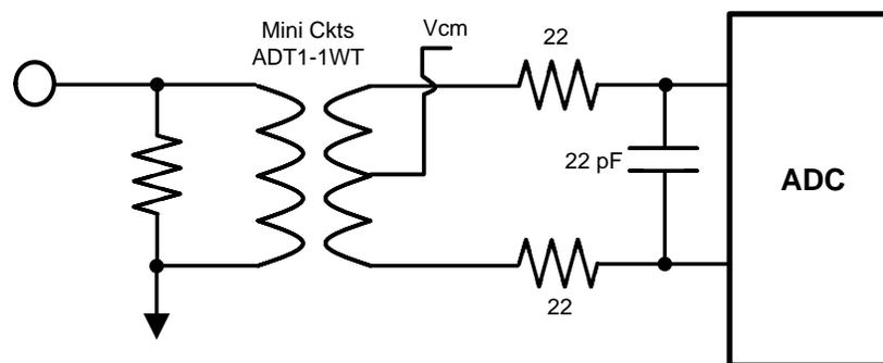
**Figure 1. Transformer Drive Circuit**
