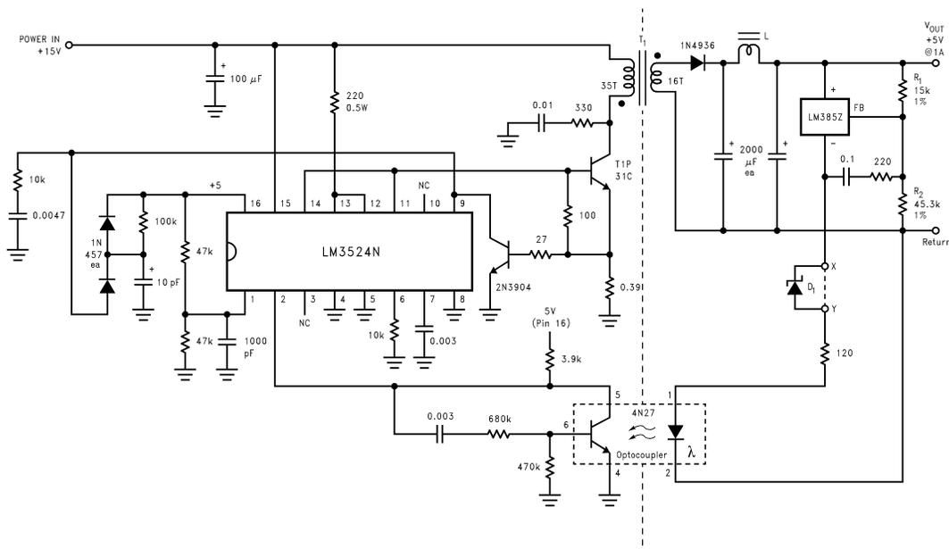
L = 15 turns #22 wire wrapped on ½W resistor body.
