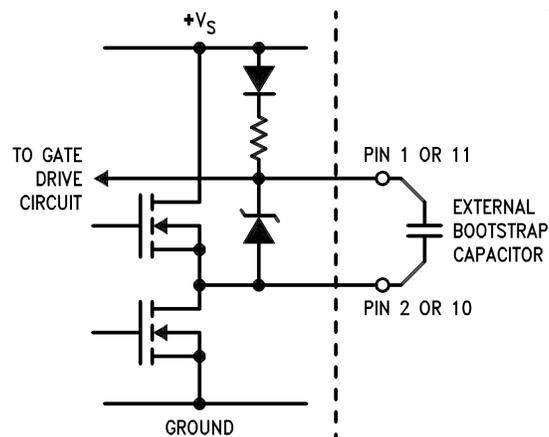
Figure 7. Use of External Bootstrap Capacitors (b)
