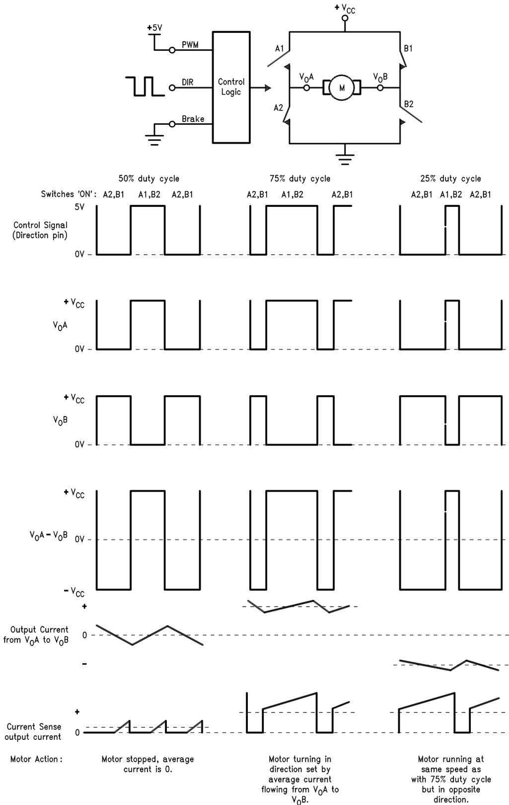
Figure 9. Idealized Switching Waveforms for Locked Antiphase Control
