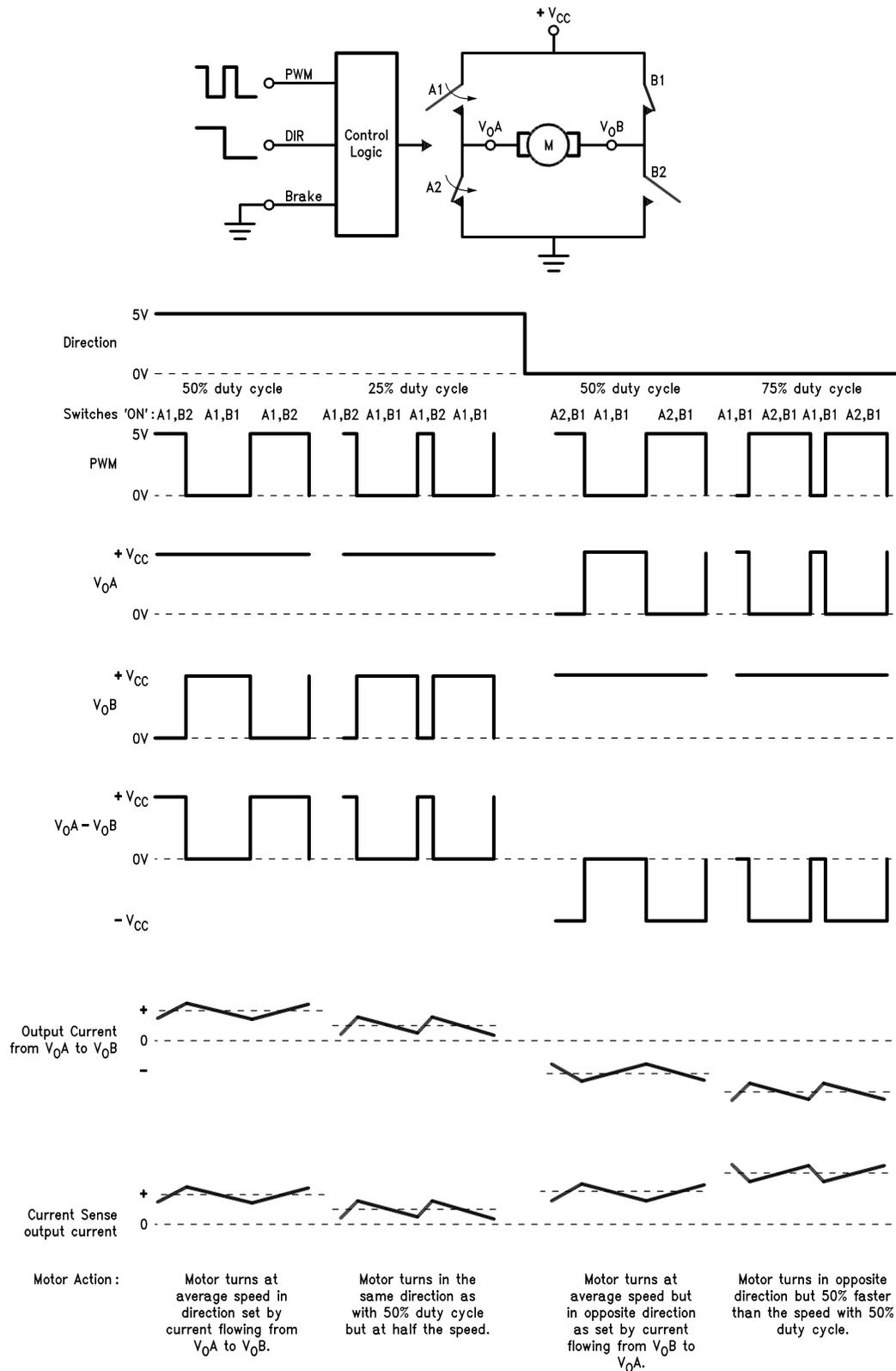
Figure 10. Idealized Switching Waveforms for Sign/Magnitude Control
