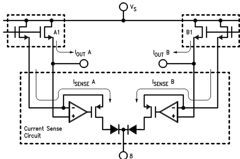
**Figure 5. The Current Sensing Circuitry of the LMD18200**
