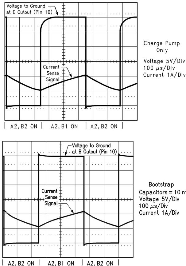
**Figure 8. Comparison of Switching Waveforms with and without the Use of Bootstrap Capacitors**
