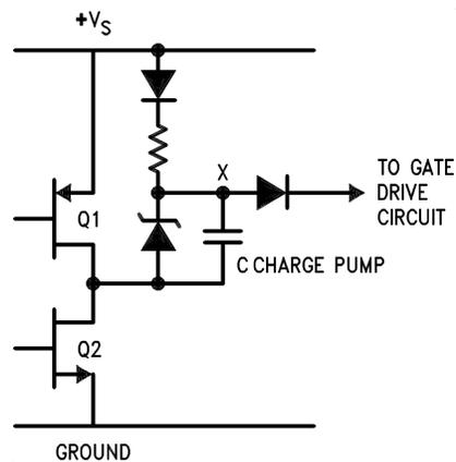
Figure 6. Internal Charge Pump Used in the LMD18200 (a)
