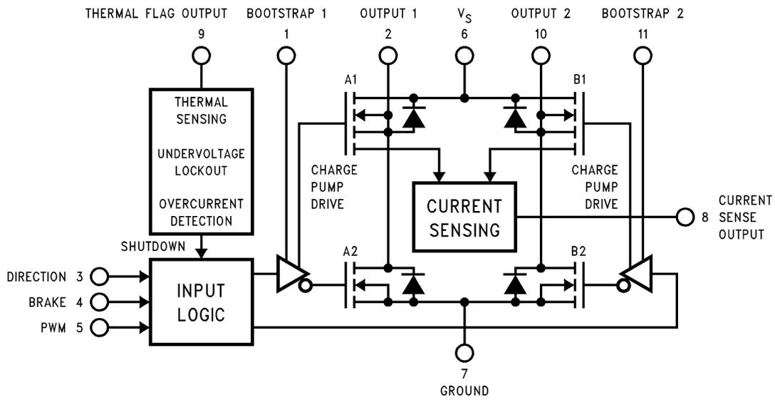
Figure 2. Block Diagram of the LMD18200
