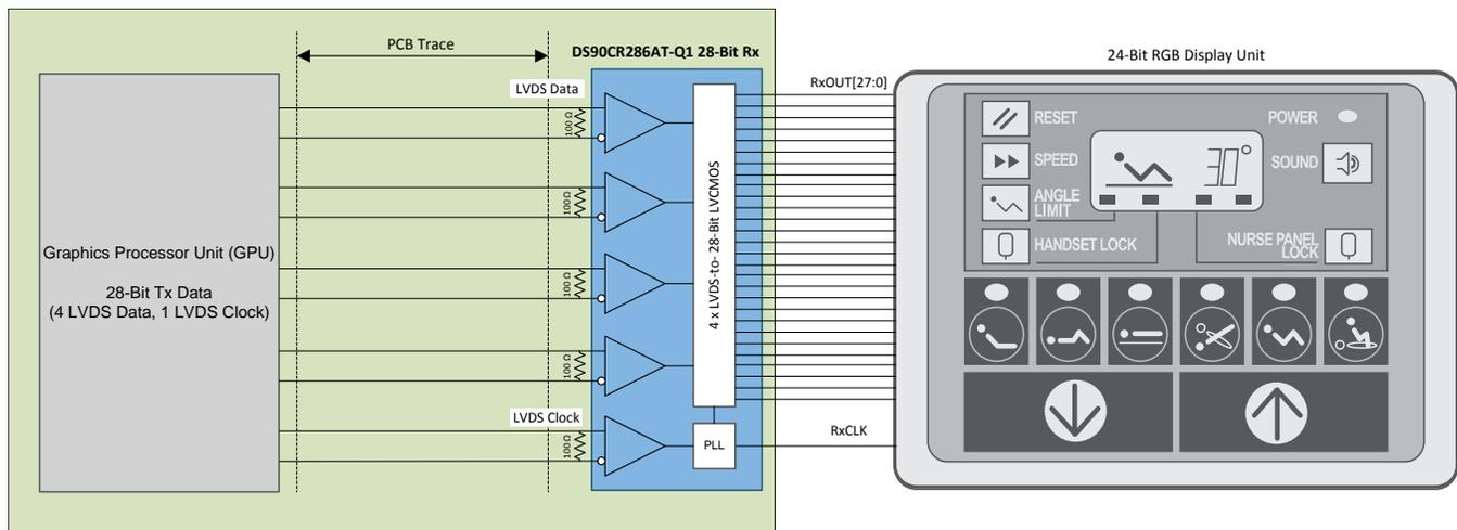
Figure 8. GPU Connection Diagram to DS90CR286AT-Q1 Receiver
