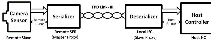
**Figure 1. Typical FPD-Link III Connection with I<sup>2</sup>C Bus**
