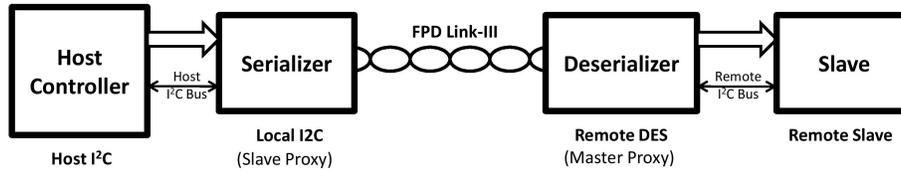
Figure 7. I<sup>2</sup>C Master attached to Serializer
