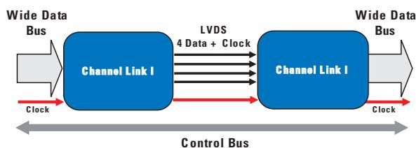
**Figure 1. Early Serializers Converted a Wide Bus to Four Data Lanes and a Clock**
