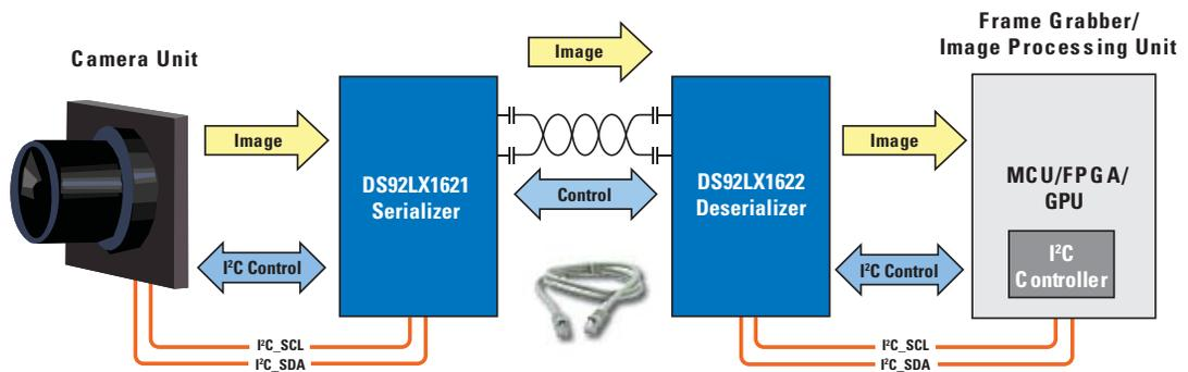
Figure 3. Camera Application, 16-Bit LVCMOS Bus and Embedded I<sup>2</sup>C Compatible Control
