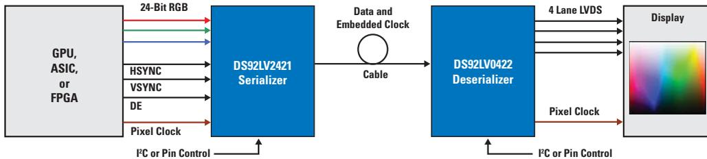
**Figure 5. Format Conversion with Channel Link II and III SerDes**
