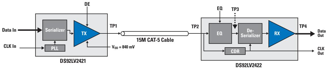
Figure 2. Channel Link II SerDes I/O Block Diagram and Test Case
