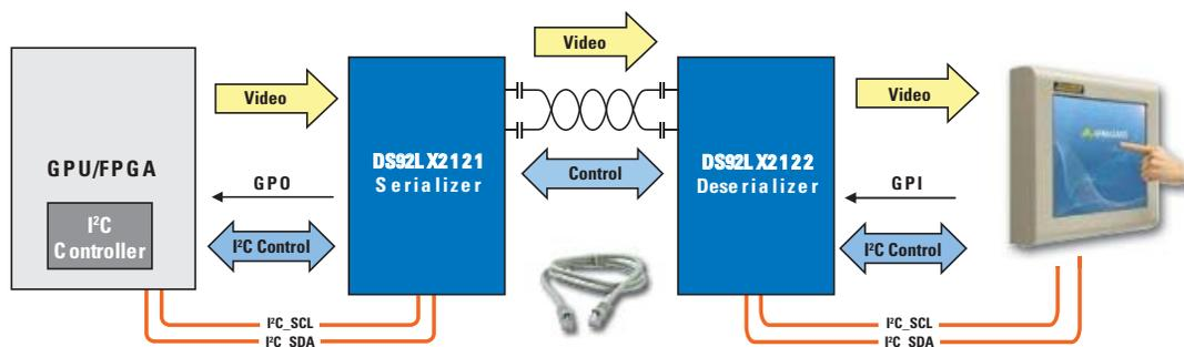
Figure 4. Display Application, 21-Bit LVCMOS Bus and Embedded I<sup>2</sup>C Compatible Control
