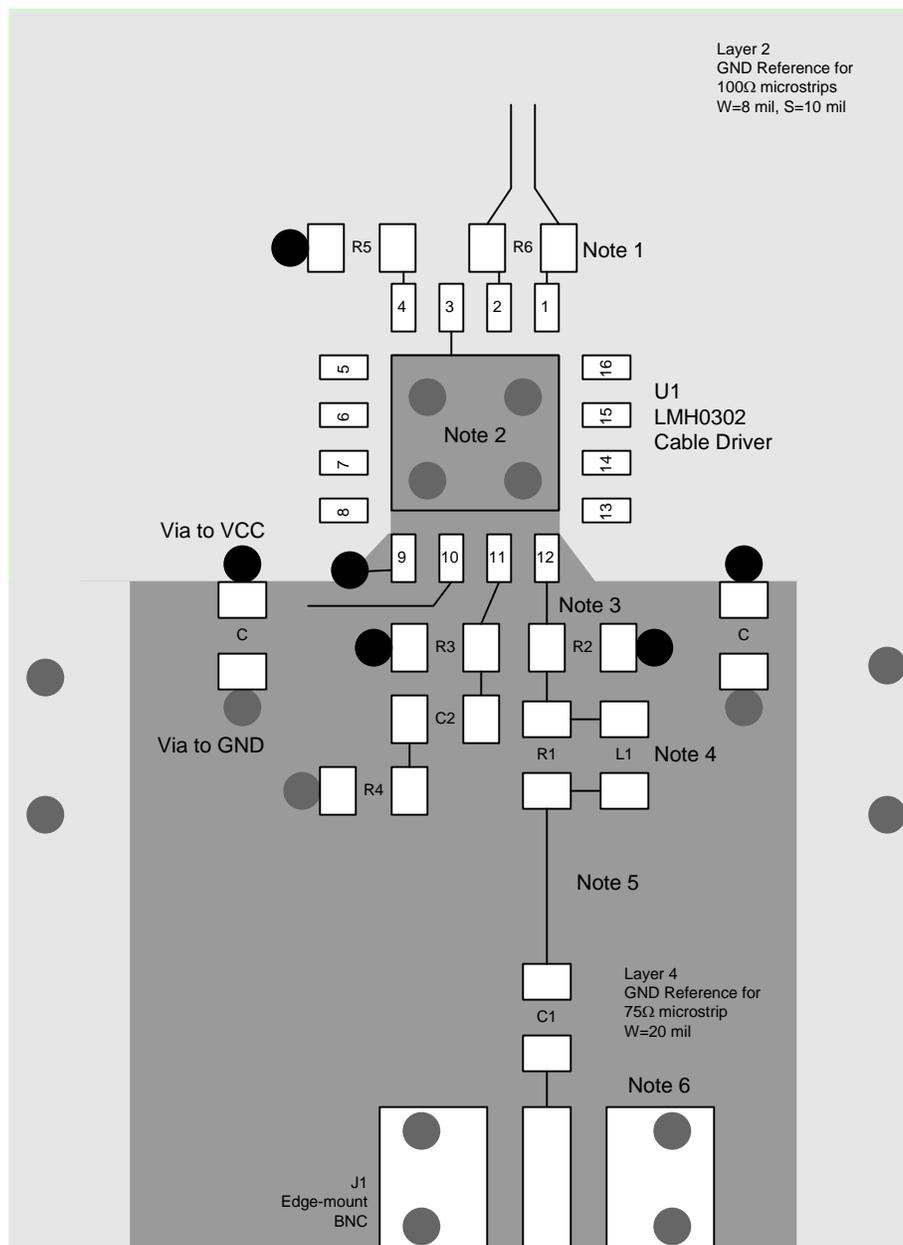
**Figure 7. Layout Recommendations For The LMH0302 Cable Driver (Showing Signal Path And Power Hook-Up)**
