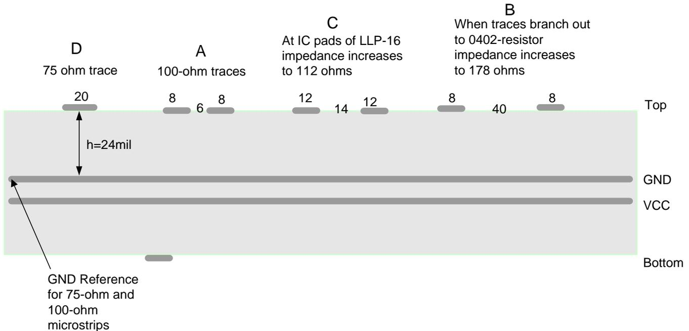
Figure 2. Stack-up example with one ground reference for 75Ω and 100Ω traces
