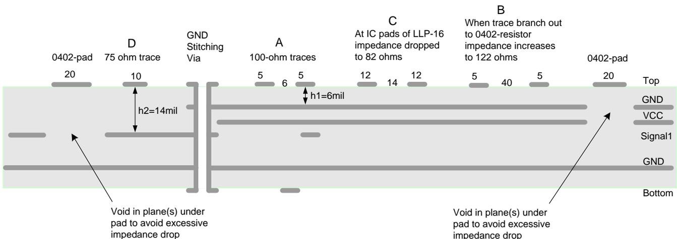
Figure 4. Stack-Up Example With Fine Trace That May Require Ground Relief Under Pads
