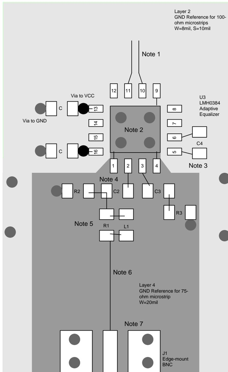
**Figure 9. Layout Recommendations For The LMH0384 Adaptive Equalizer (Showing Signal Path And Power Hook-Up)**
