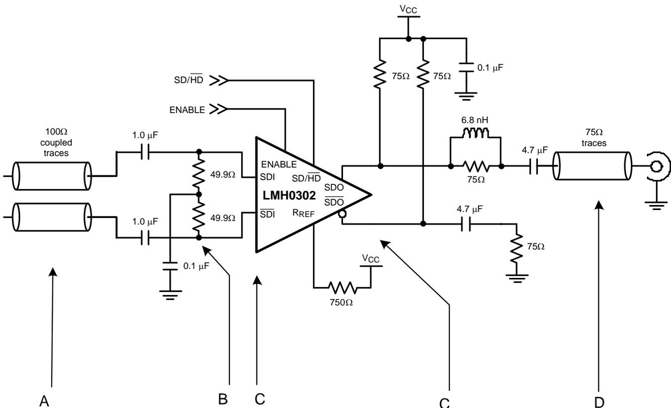
**Figure 1. Schematic Diagram of the LMH0302 Cable Driver**
