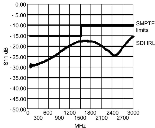
**Figure 5. Plot Of Input Return Loss (IRL) of an SDI Port and SMPTE Limits**
