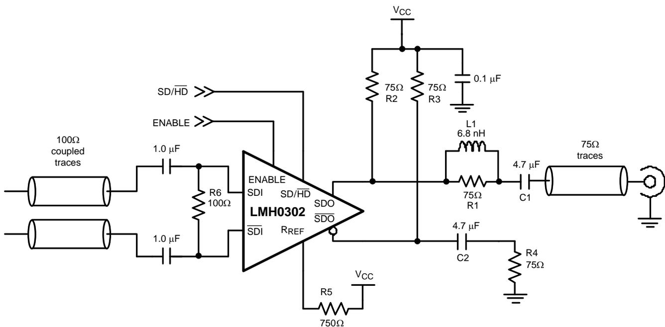
Figure 6. Schematic Diagram of the LMH0302 Cable Driver
