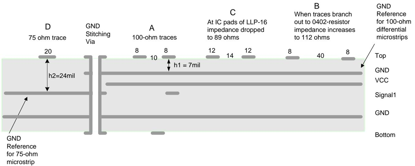
Figure 3. Stack-Up Example With Separate Ground Reference For 75Ω And 100Ω Traces
