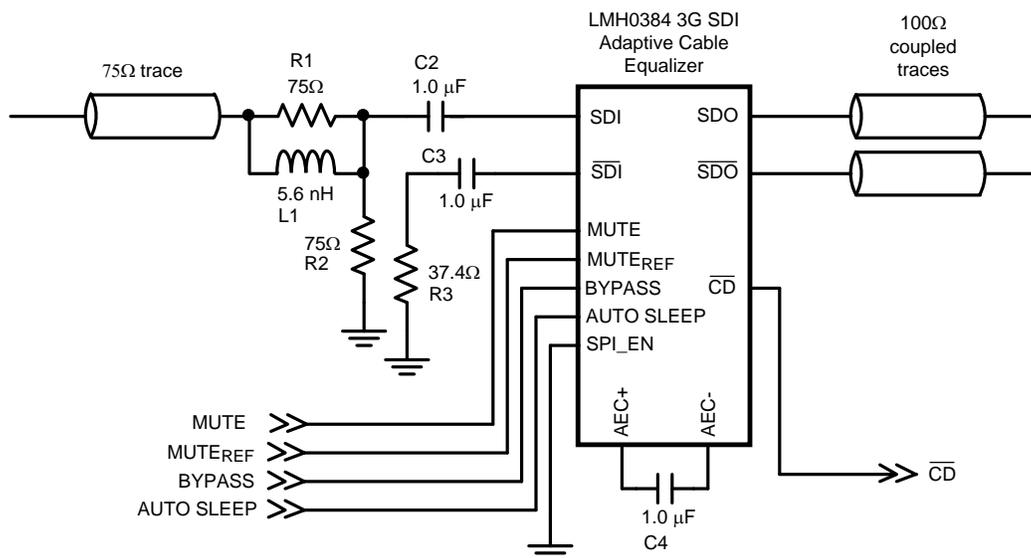
Figure 8. Schematic Diagram of the LMH0384 Adaptive Equalizer
