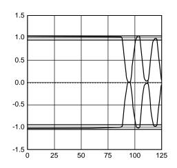
Figure 14. 100 Mb/s Vod with 33 nf Blocking Capacitors
