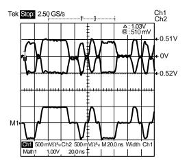
Figure 3. Sample 100 Mb/s Waveform (MLT-3)
