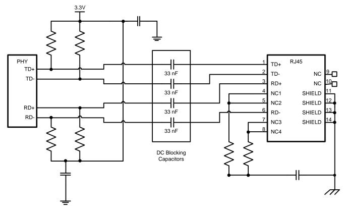
Figure 5. Transformerless Configuration
