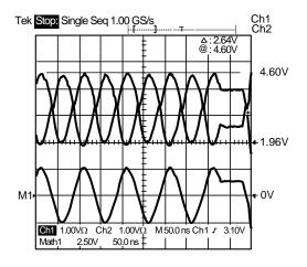
Figure 7. Sample 10 Mb/s Waveform
