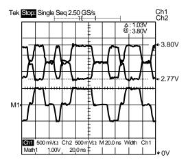
Figure 6. Sample 100 Mb/s Waveform
