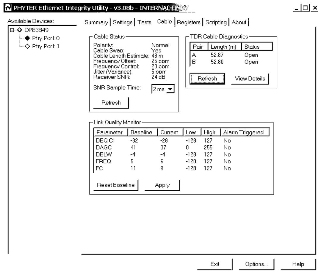
Figure 11. Integrity Utility-Cable Tab
