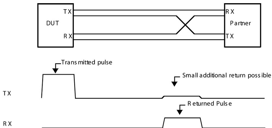
**Figure 6. TX-/RX+ Cross-Wired Circuit (into Inactive or Unpowered Partner)**
