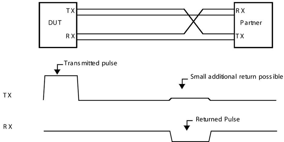
Figure 7. TX+/RX+ Cross-Wired Circuit (into Inactive or Unpowered Partner)
