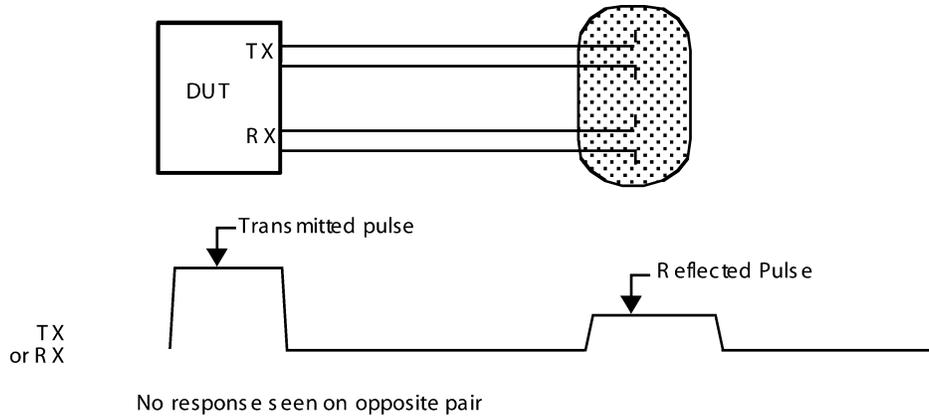
Figure 3. Open Circuit
