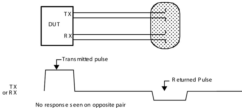
Figure 4. Short Circuit Within a Single Pair
