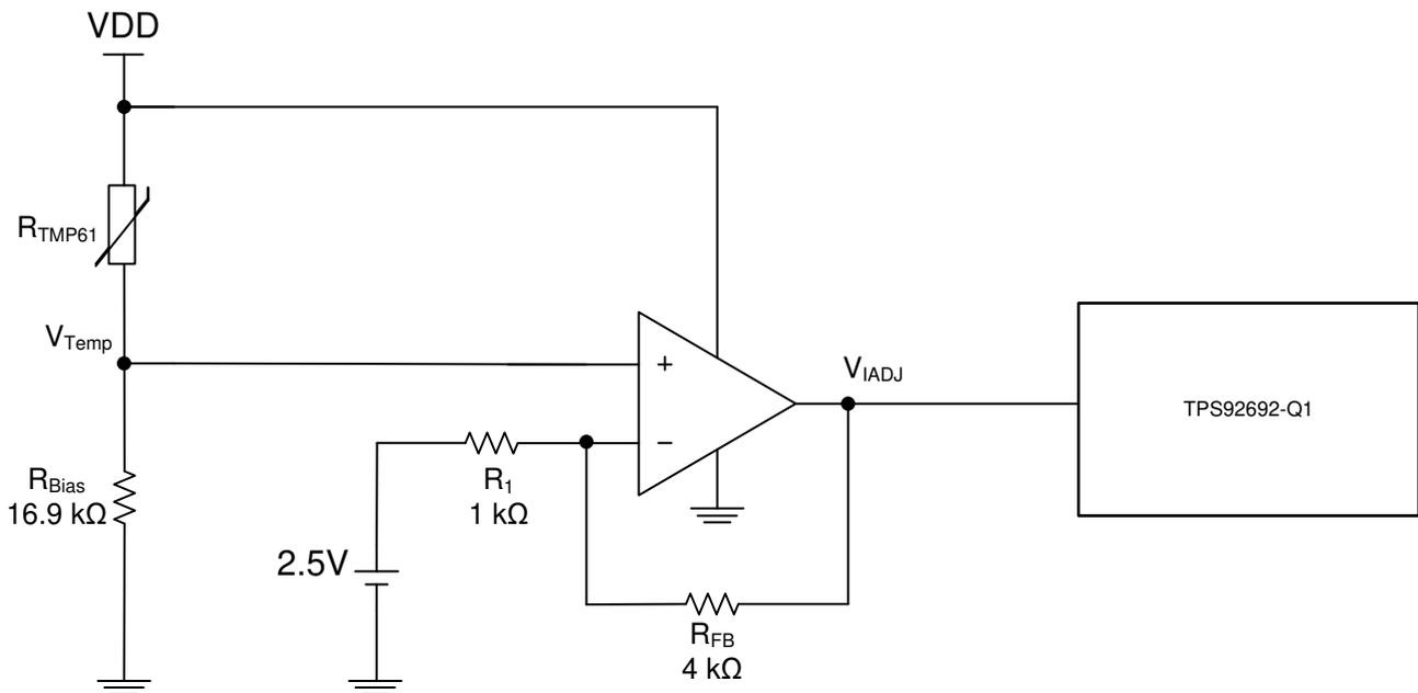
Figure 7. Voltage Divider With TMP61-Q1 Thermistor and Op Amp
