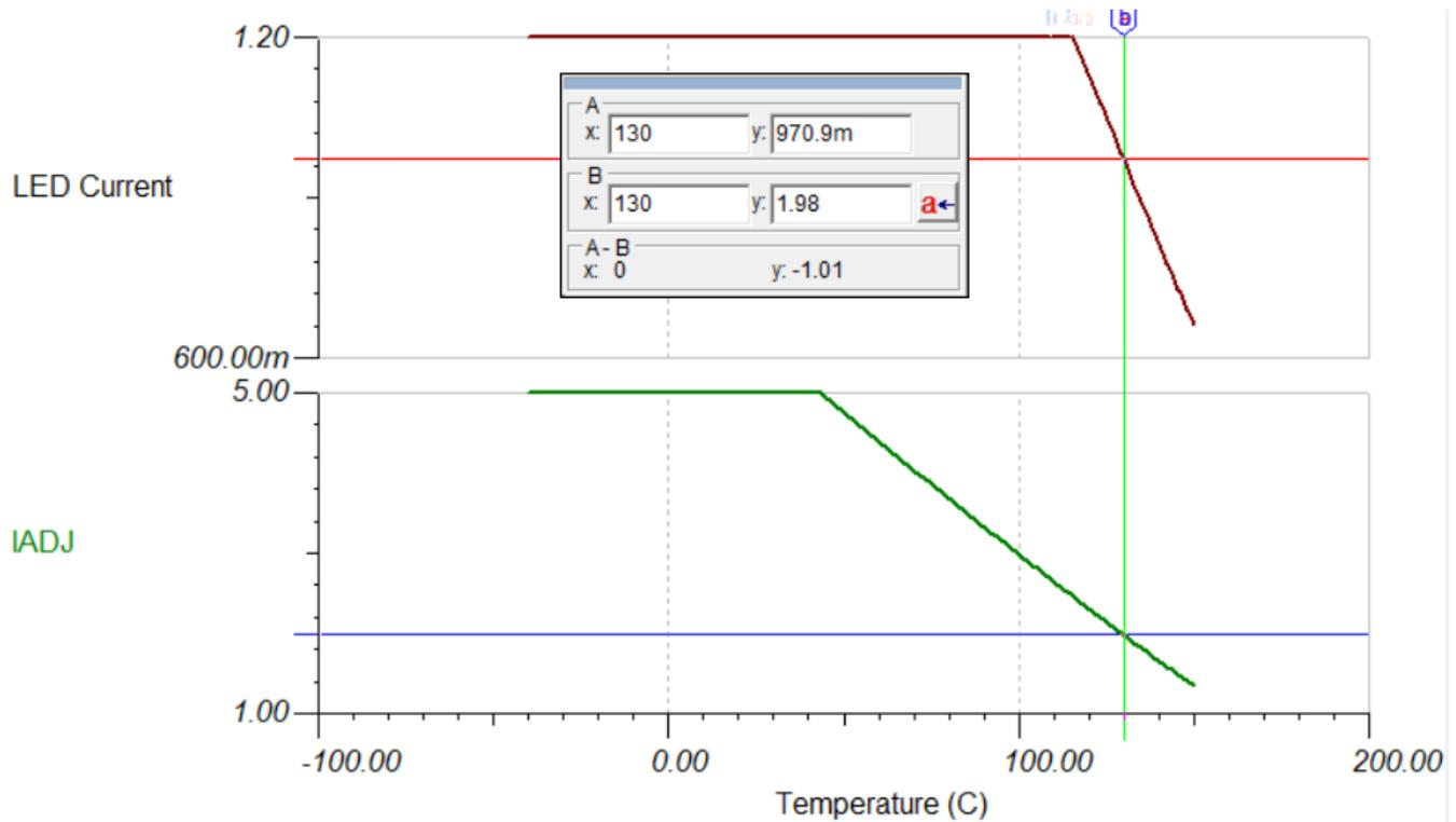
Figure 9. 130 °C Output Current Curve
