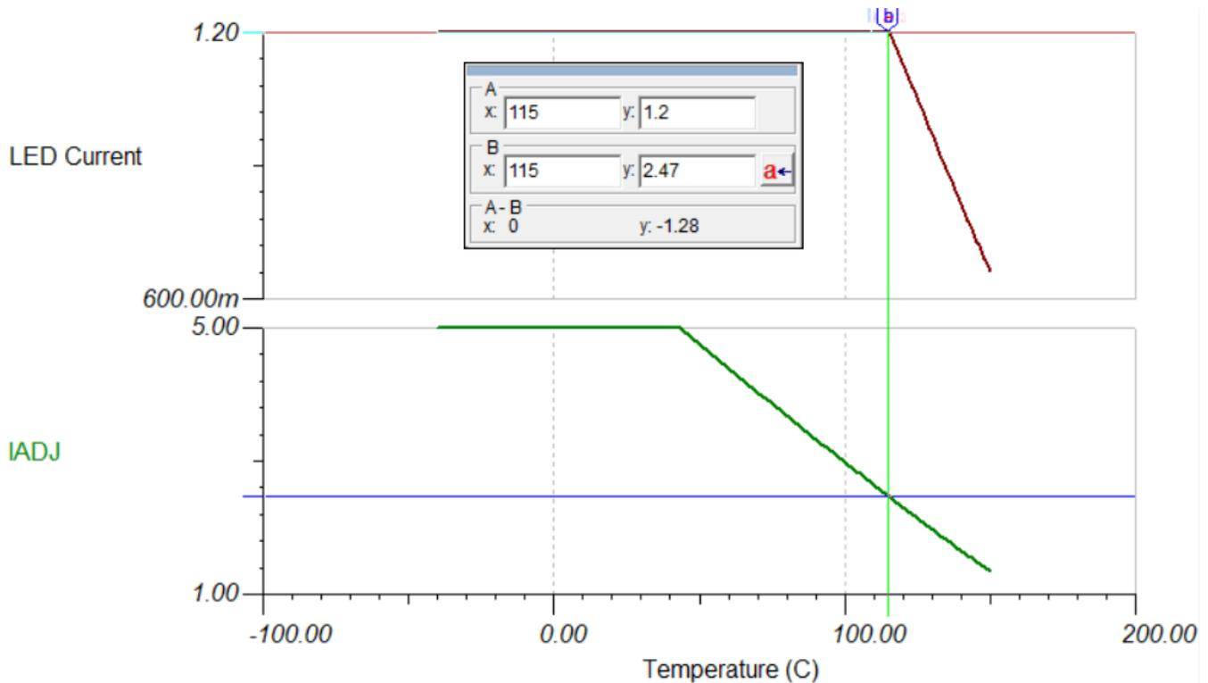
Figure 8. 115 °C Output Current Curve
