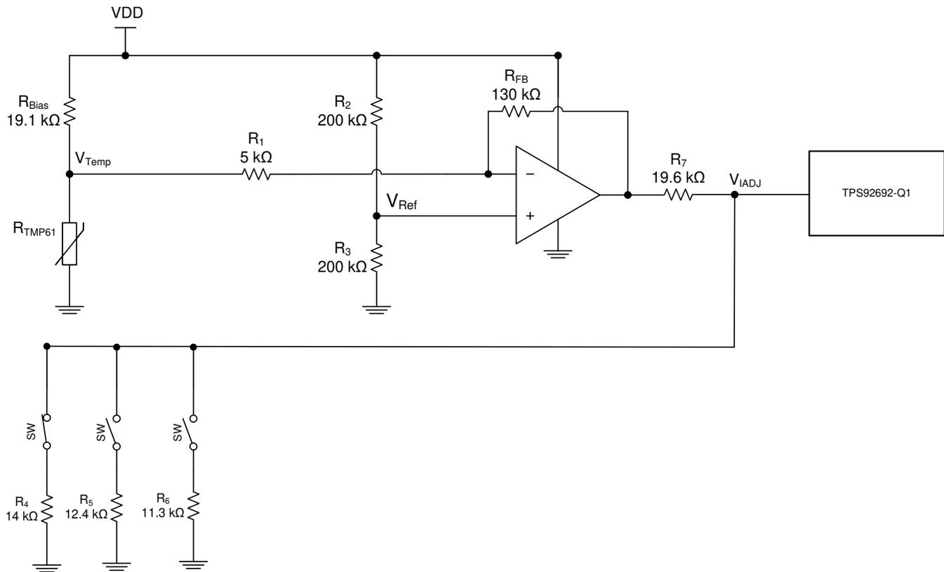
**Figure 10. Voltage Divider With TMP61-Q1 Thermistor, Op Amp, and Binning Resistors**
