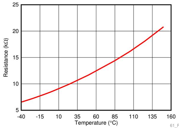
**Figure 1. TMP61-Q1 Resistance Curve vs Temperature**
