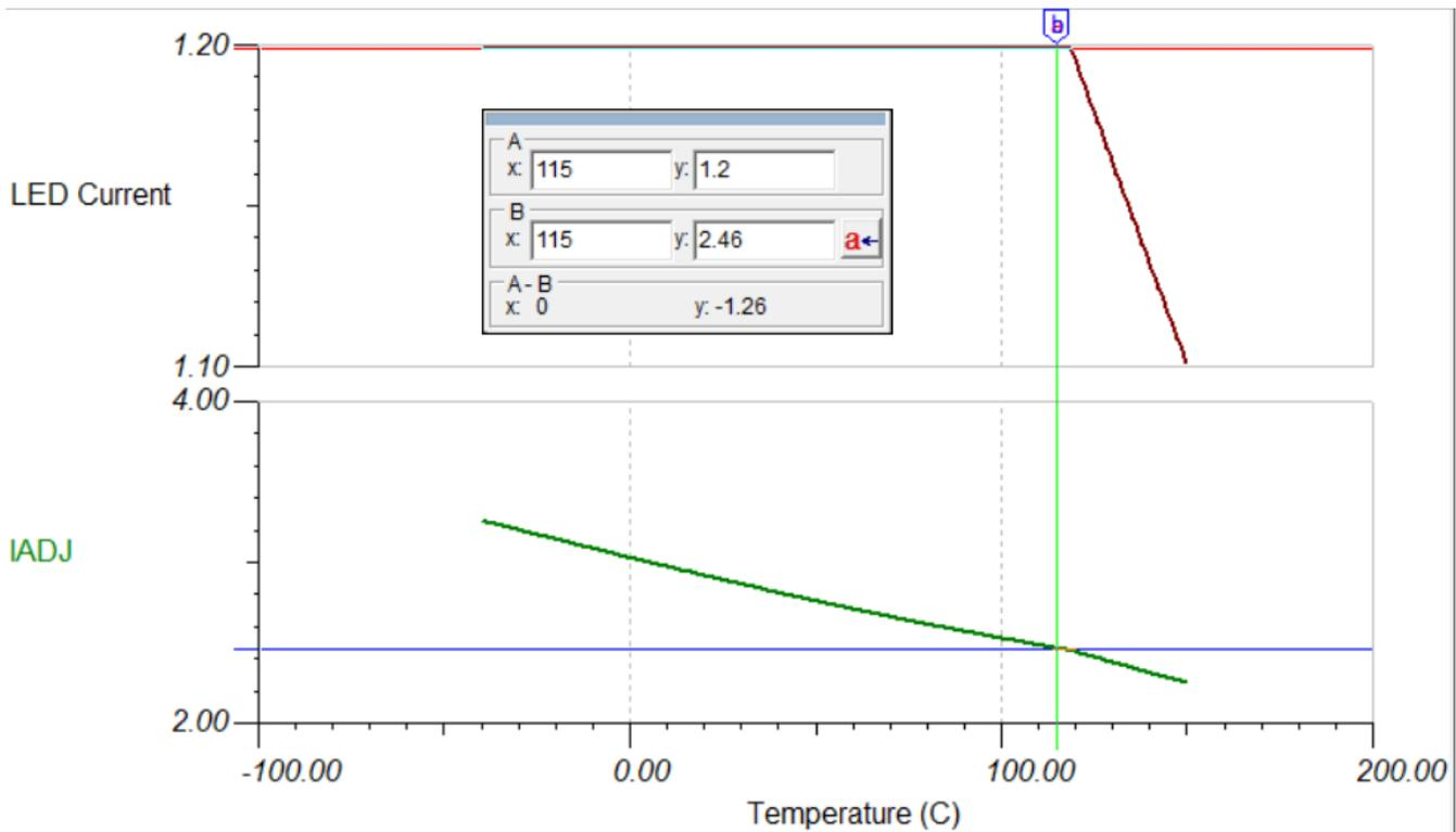
**Figure 5. LED Output Current vs Temperature**
