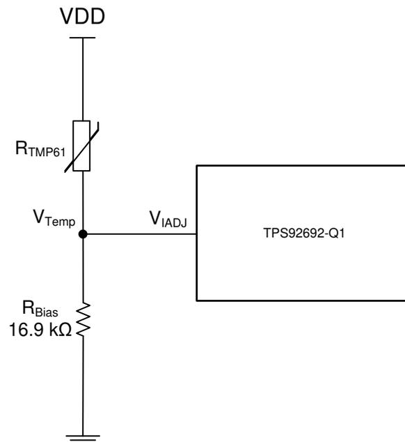
Figure 4. Voltage Divider With TMP61-Q1
