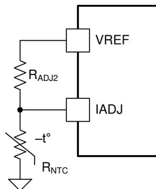
**Figure 2. TPS92692-Q1 Functional Diagram NTC Thermistor Schematic**
