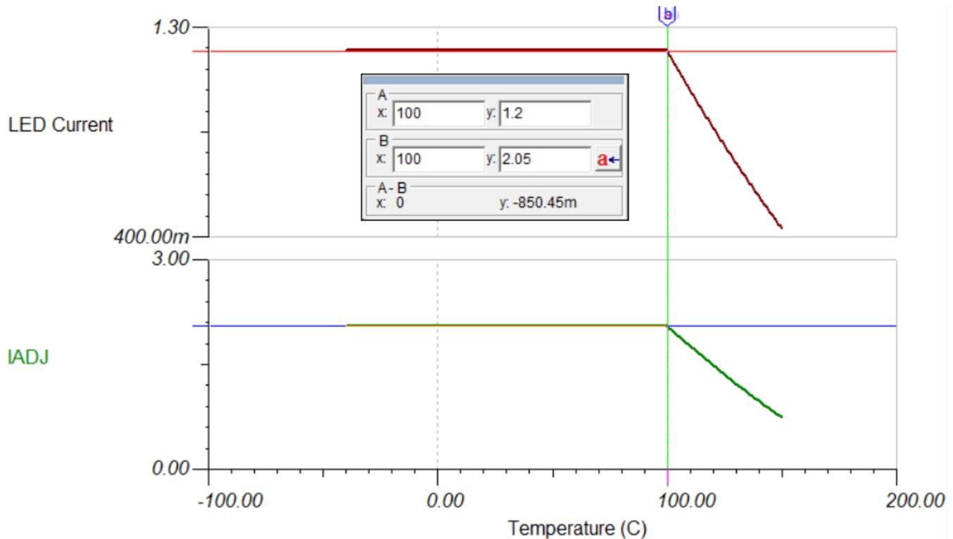
Figure 11. 100 °C Current Output Curve
