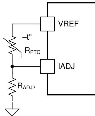
Figure 3. TPS92692-Q1 Functional Diagram PTC Schematic
