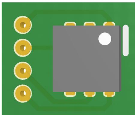
**Figure 8. TMP117 Mini Probe Board Top Side L3**
