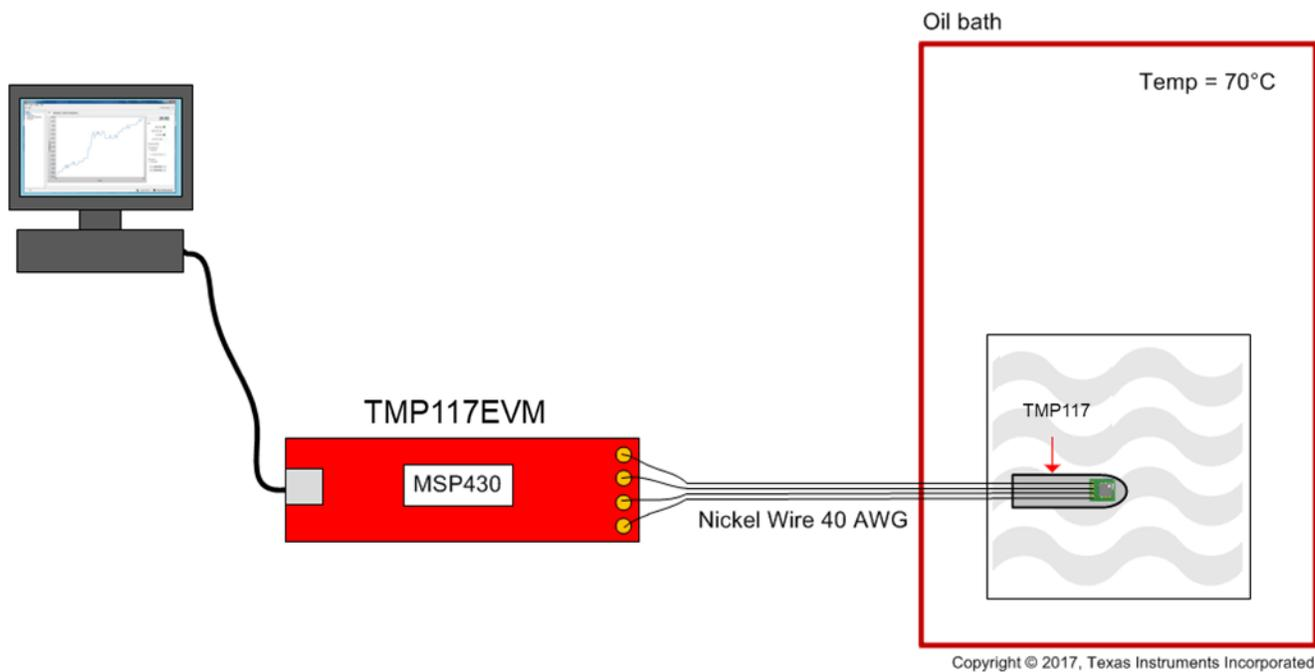
**Figure 20. Stirred Oil Thermal Response Measurement System**
