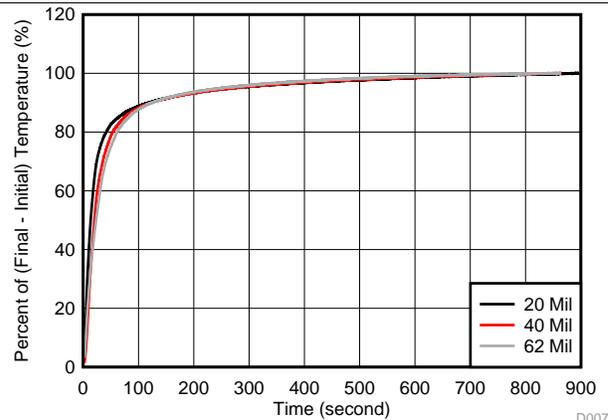
**Figure 25. Armpit Thermal Response With Different Board Thickness**
