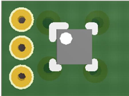
**Figure 6. Small LMT70 Probe Board Top Side**
