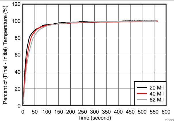
**Figure 24. Oral Thermal Response With Different Board Thickness**
