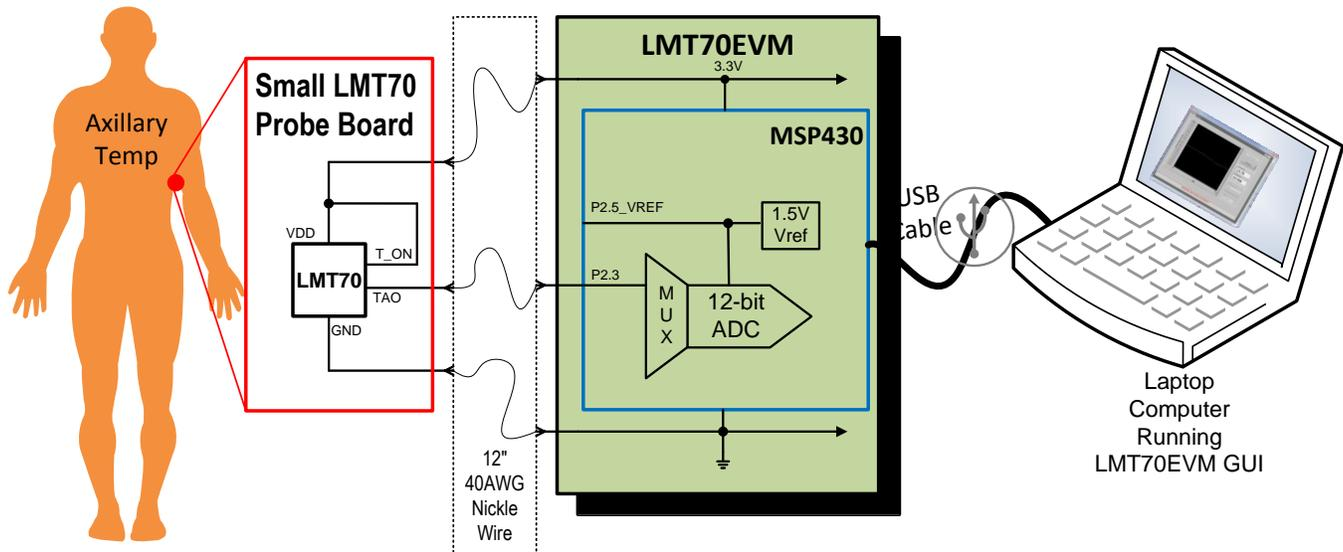
**Figure 16. LMT70 Probe Board Thermal Response Measurement System**
