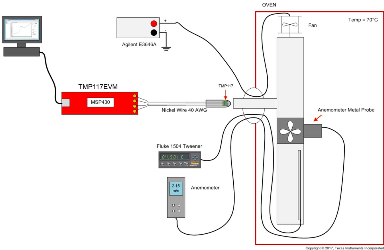
**Figure 19. Moving Air Thermal Response Measurement System**
