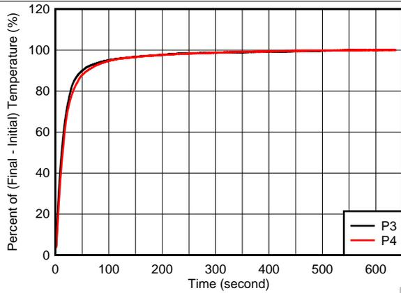
**Figure 22. Oral Thermal Response With (P4) And Without (P3) Thermal Pad Soldered**
