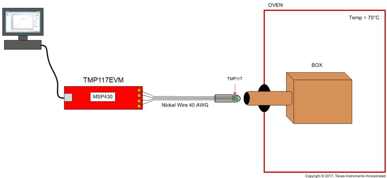
**Figure 18. Still Air Thermal Response Measurement System**
