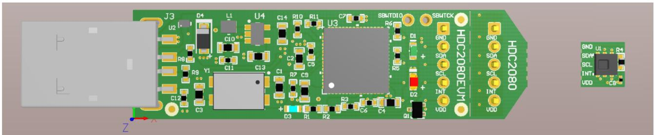
**Figure 13. HDC2080EVM : PC Interface and Smaller Sensor Module**
