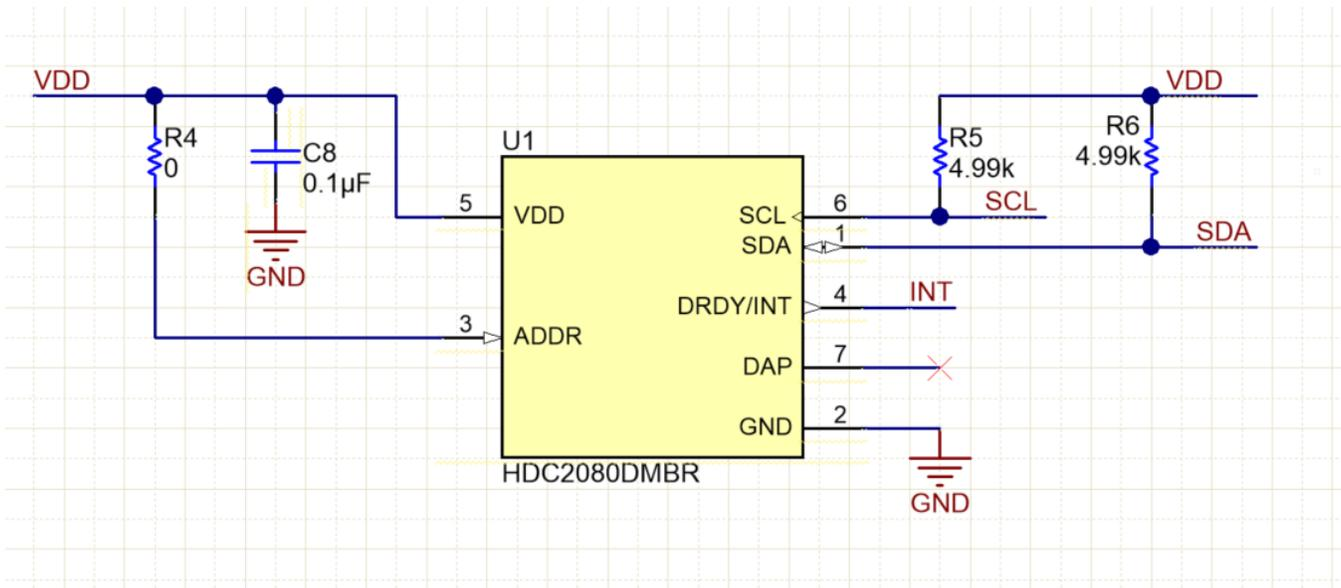
Figure 2. HDC2080EVM : Sensor Module
