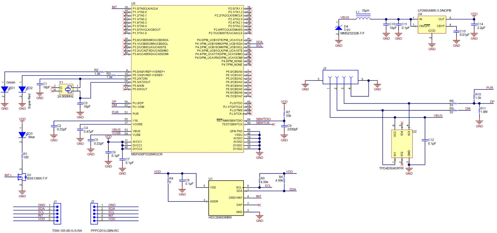
Figure 56. HDC2080EVM Schematic
