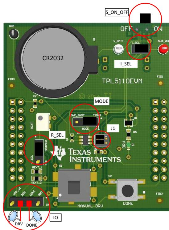
Figure 7. Jumpers Configuration – EVM Standalone Without Microcontroller
