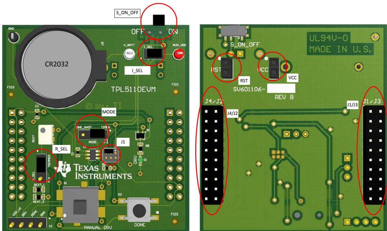
**Figure 9. Jumpers Configuration – EVM With LaunchPad**
