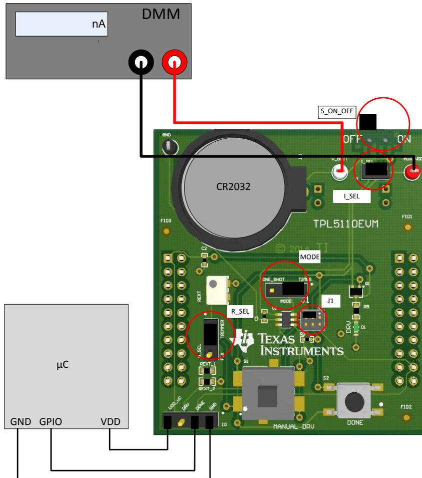
Figure 12. Current Measurement Setup – TPL5110 With Microcontroller
