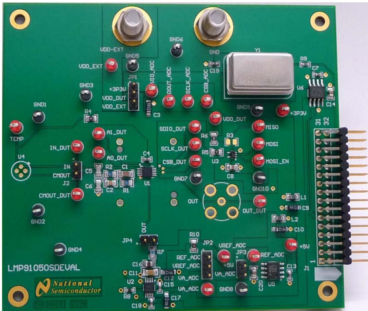
Figure 2 – LMP91050 Evaluation Board Assembly
