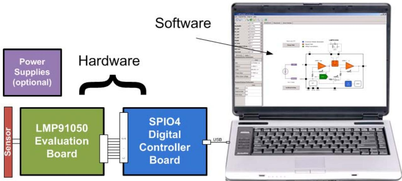
Figure 1 – Connection Diagram
