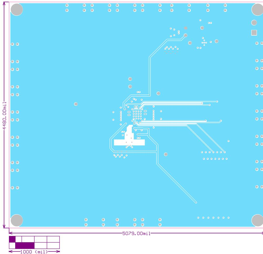
**Figure 8: Internal Power Plane, Layer #3 (Not to scale)**
