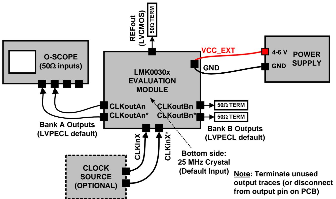
Figure 2: LMK00306 Evaluation Board Quick Start Setup
