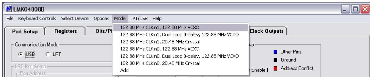
**Figure 5: Setting the Default mode for LMK04808**
