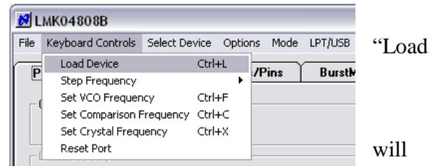
**Figure 4 – Loading the Device**
