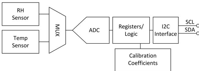
**Figure 3. Relative Humidity and Temperature Sensor Block Diagram**
