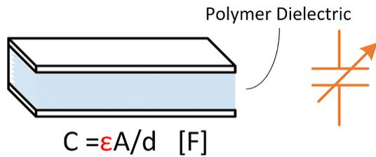
**Figure 2. Capacitor With Polymer Dielectric**
