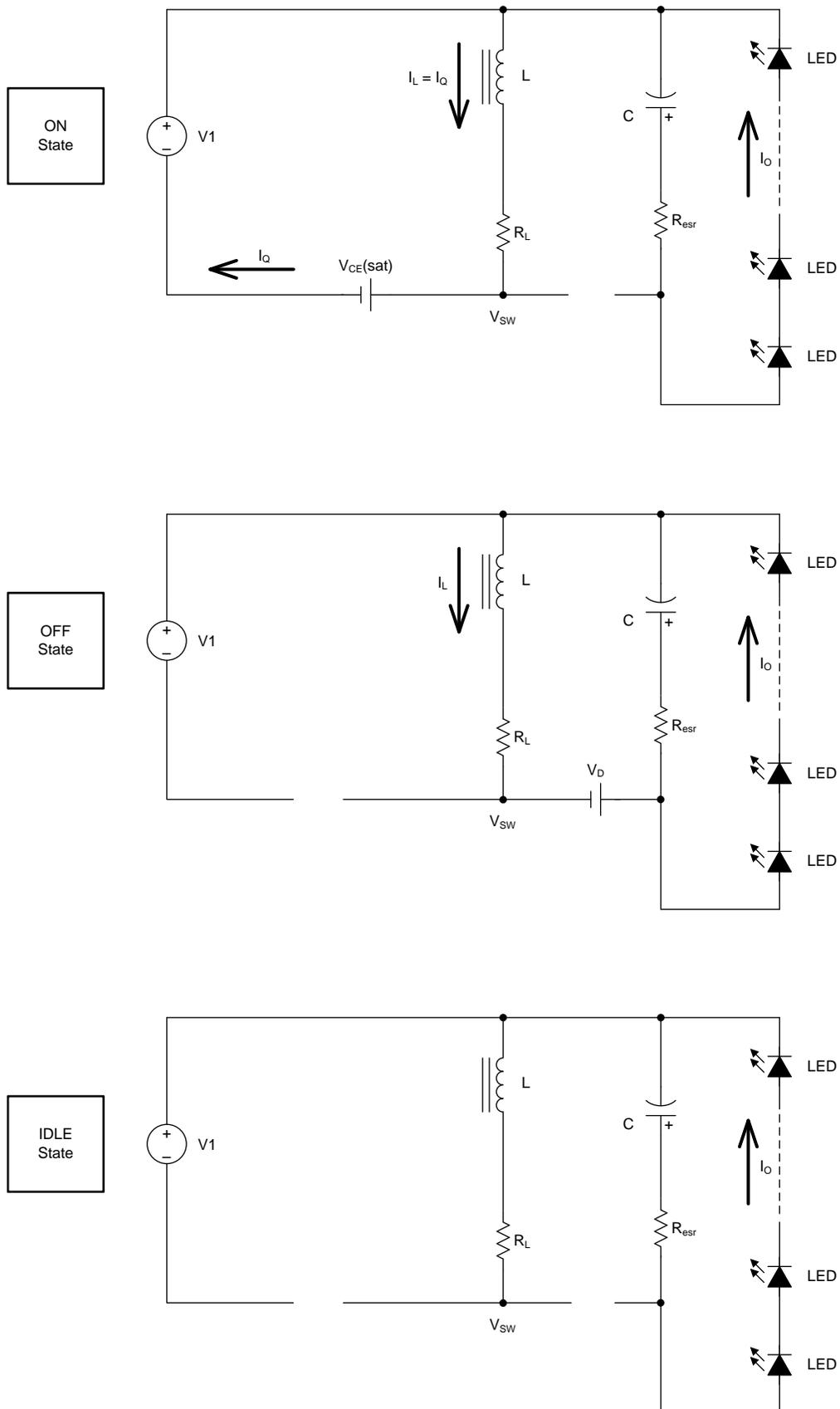
Figure 2. Buck-Boost Power Stages in Discontinuous Mode
