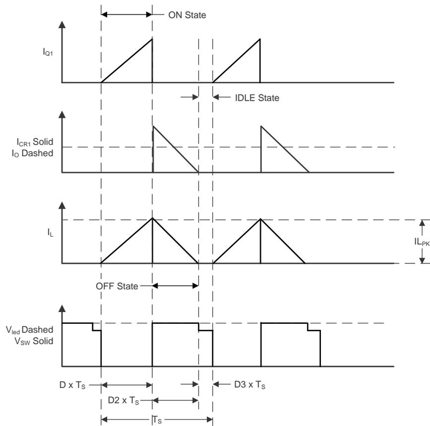
**Figure 3. Discontinuous Mode Power Stage Buck-Boost Wave Forms**
