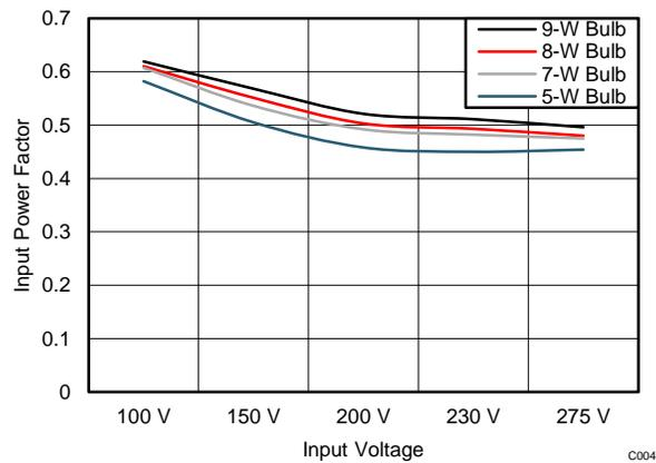
**Figure 9. Input Power Factor vs V<sub>IN</sub>**
