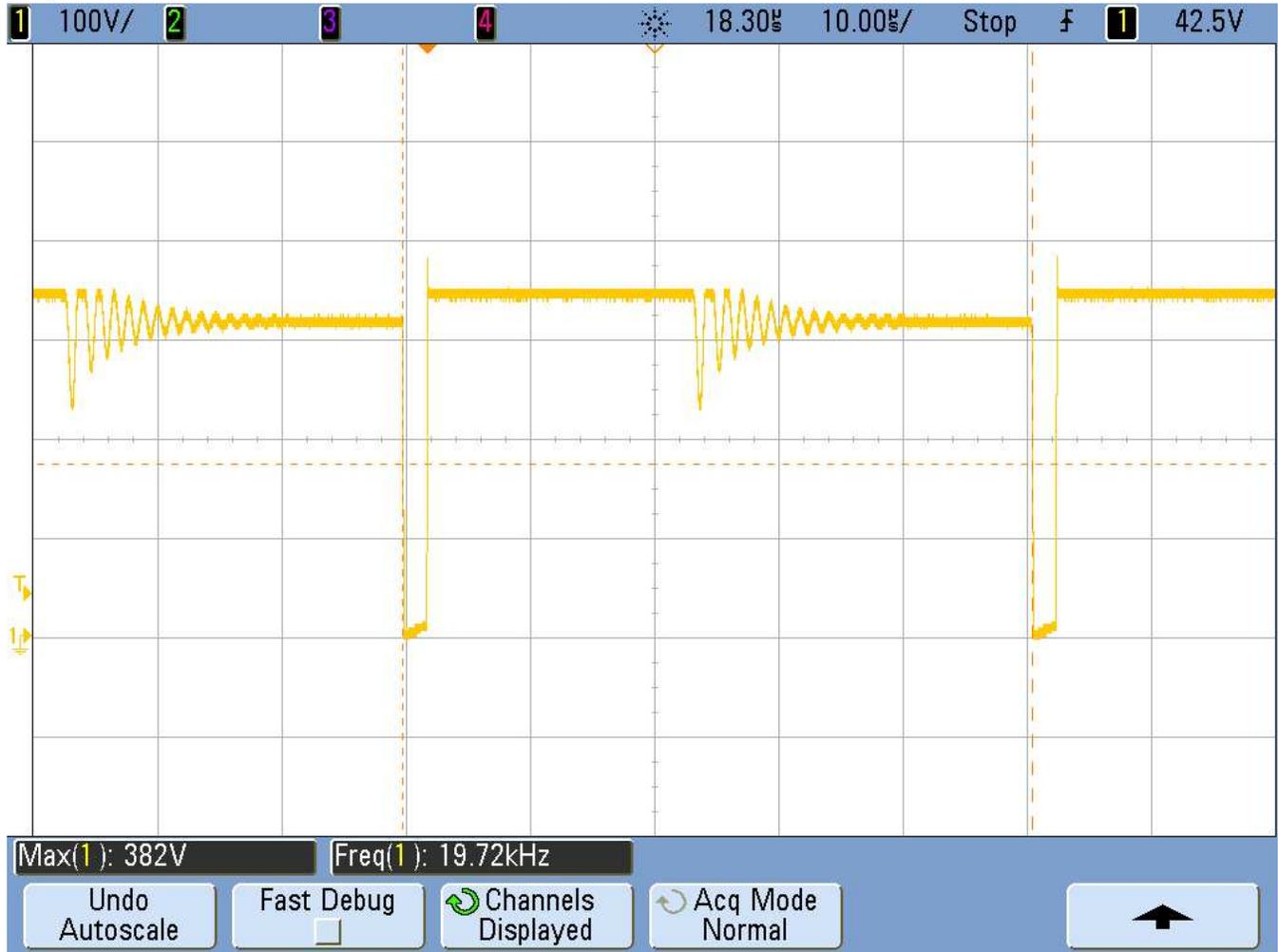
Figure 10. SW Node Waveform at  $V_{IN} = 230 V_{AC}$  for a 5 W Bulb
