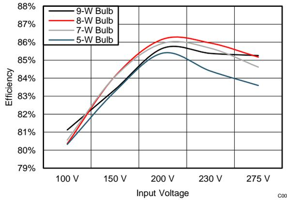
**Figure 6. Efficiency vs V<sub>IN</sub>**
