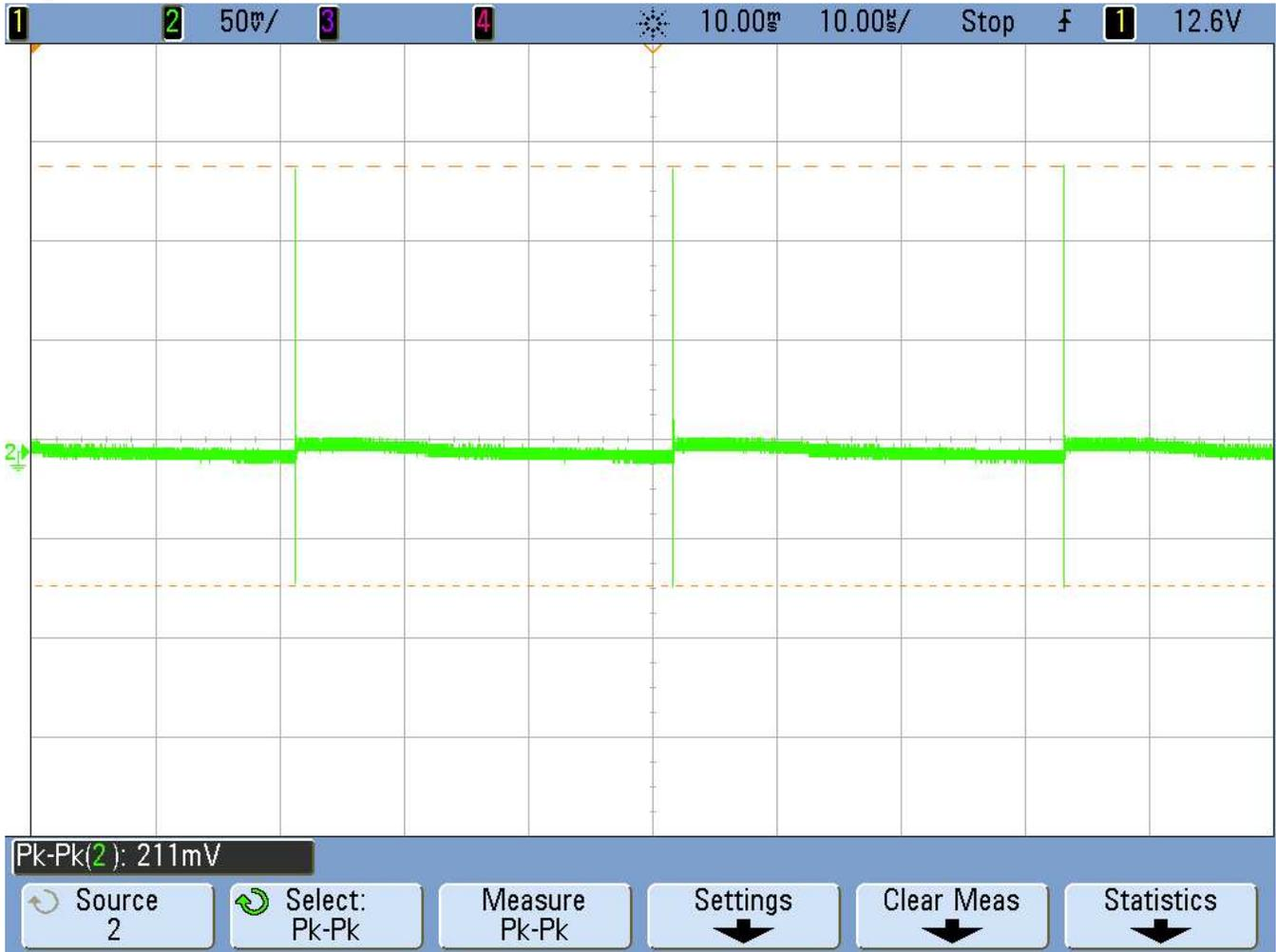
Figure 16. V<sub>OUT</sub> Ripple at V<sub>IN</sub> = 230 V<sub>AC</sub> for a 8 W LED Bulb
