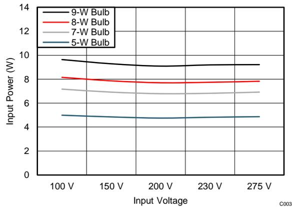
**Figure 8. Input Power vs V<sub>IN</sub>**
