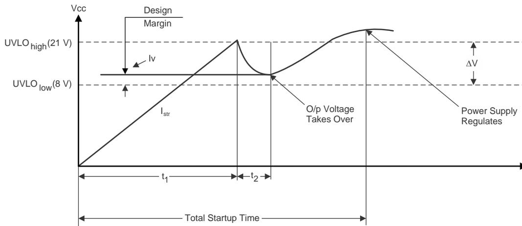
**Figure 4. Timing Diagram of Startup Sequence in UCC28722**
