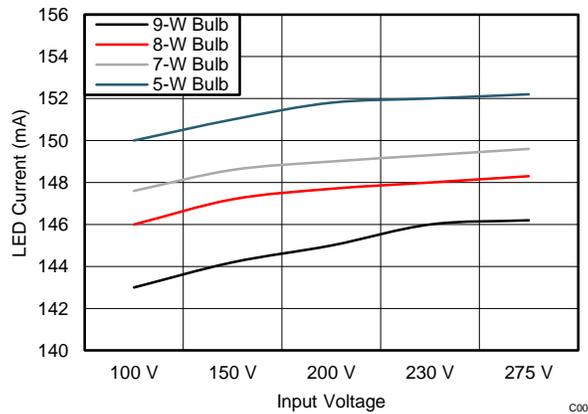
**Figure 7. Line Regulation vs V<sub>IN</sub>**
