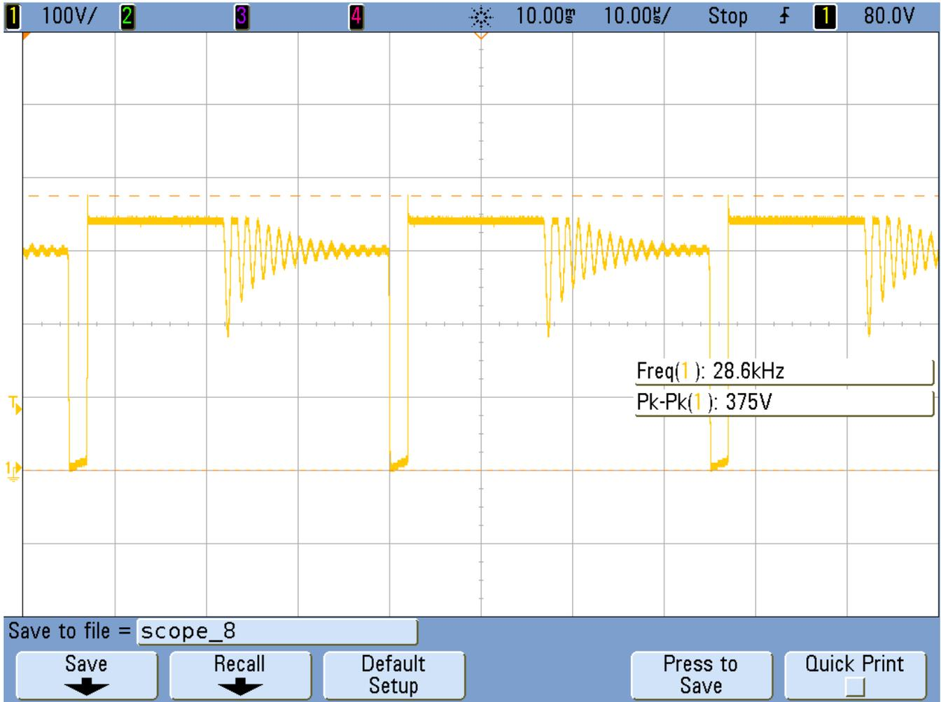
Figure 11. SW Node Waveform at  $V_{IN} = 230 V_{AC}$  for a 7 W Bulb
