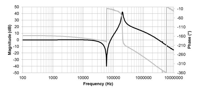
Figure 3. Measured Magnitude Response Using Component Values In Table 1
