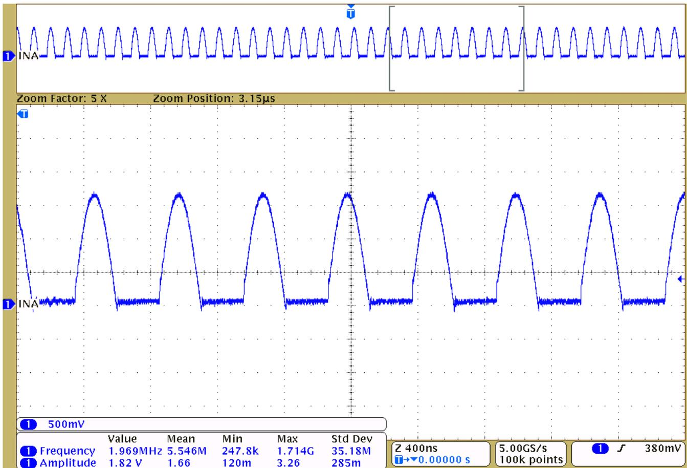
Figure 5. LDC13xx/LDC16xx Sensor Amplitude set by DRIVE\_CURRENT\_CHx
