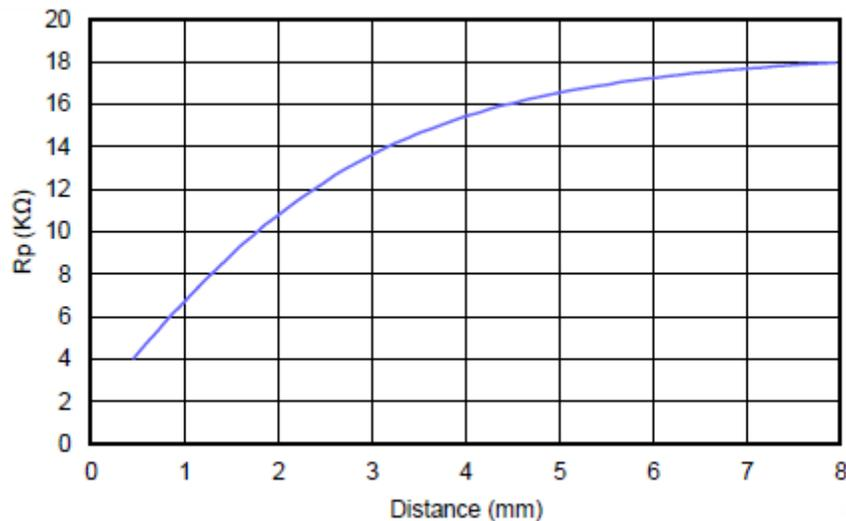
**Figure 3.  $R_p$  [k $\Omega$ ] Versus Distance [mm] of a 14-mm Diameter PCB Coil**
