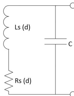
**Figure 1. Series Electrical Model of an LC Tank**
