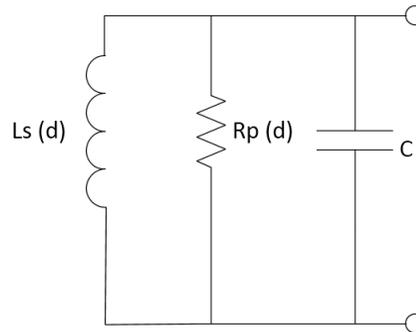
Figure 2. Parallel Electrical Model of an LC Tank
