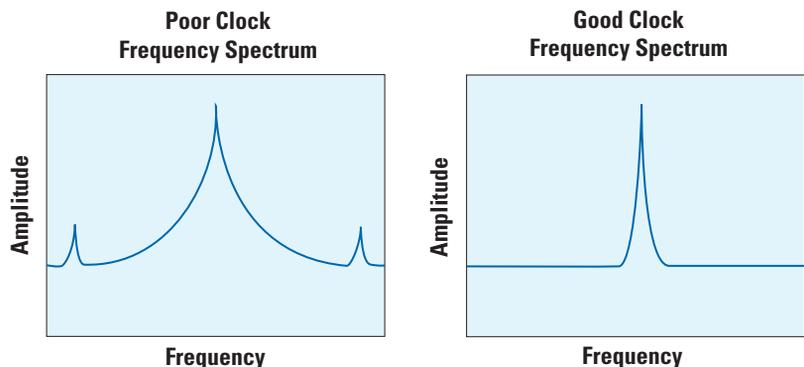
Figure 1. Examples of Clock Signal Spectral Analysis
