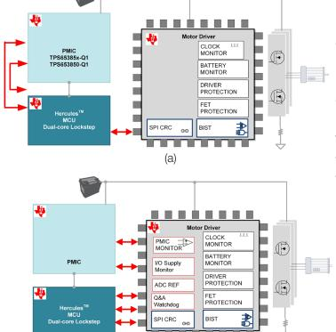
Figure 3. Illustration depicts both distributed and integrated safety concepts (a and b, respectively).
