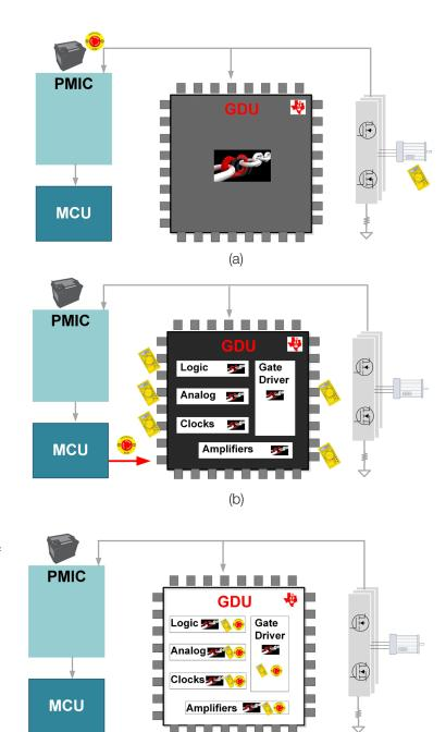
Figure 4. Common approaches to FIT rate calculation in analog components: black box, black box with a window, and white box (a, b and c, respectively).
