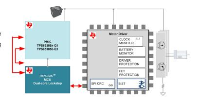
Figure 2. Random fault management for a motor driver.
