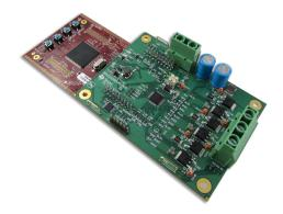
Figure 5. DRV3205-Q1 evaluation module paired with the Hercules™ MCU Launchpad development kit.
