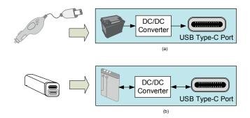
Figure 1: USB charging devices include a USB port in a car or a portable USB car charger (a); and a portable rechargeable battery/power bank (b).
