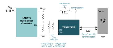
Figure 4: An USB PD power provider/charger implementation using a four-switch buck-boost and USB PD controller [8].
