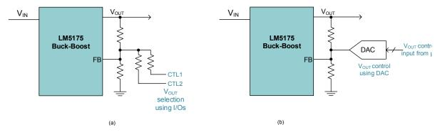
Figure 3: Resistor (a) and DAC-based (b) schemes for changing the output voltage of a four-switch buck-boost converter and or power bank (b).
