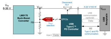
*Figure 5:* USB power provider and data implementation using a four-switch buck-boost and Type-C PD controller. controller [9], with USB data support. Using a DAC
