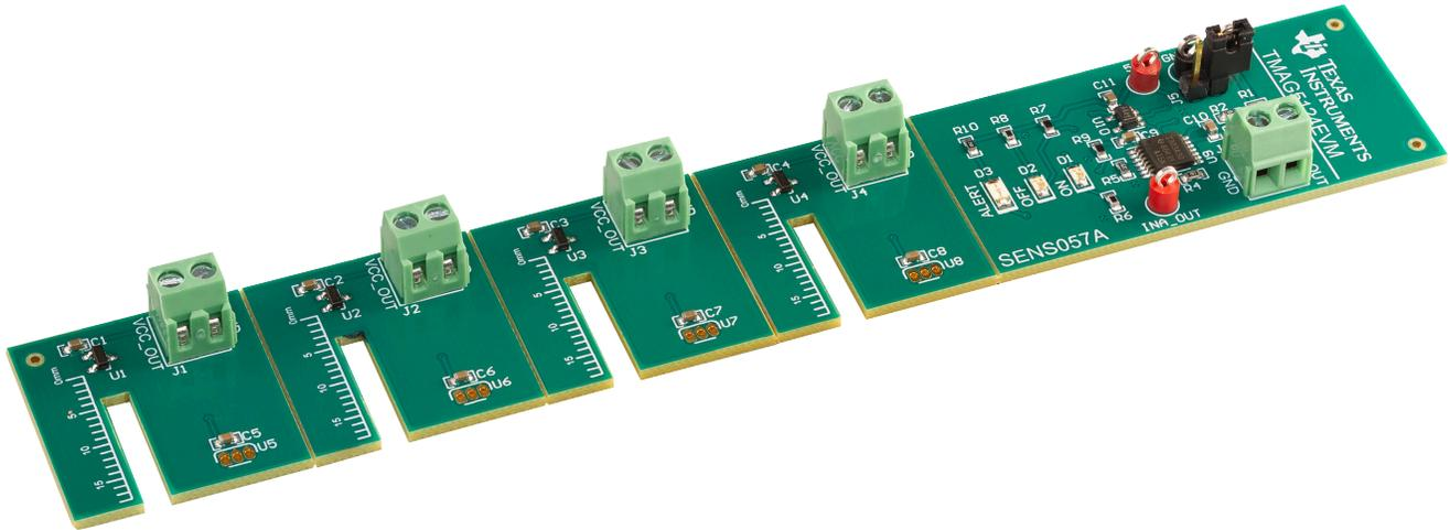
This user's guide describes the characteristics, operation, and use of the TMAG5124 2-wire evaluation module (EVM). This EVM is designed to evaluate the performance of the TMAG5124 over a separation of distance using current as the signal of interest. This document includes a schematic, printed-circuit board (PCB) layouts, and a complete bill of materials (BOM).
